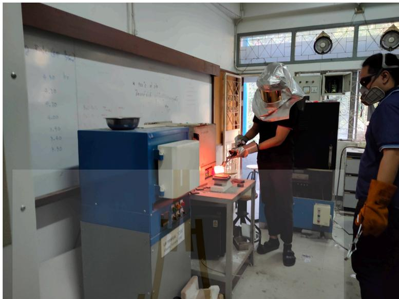
Figure A.3 Reducing the stress of the glass after melting at high temperature.
