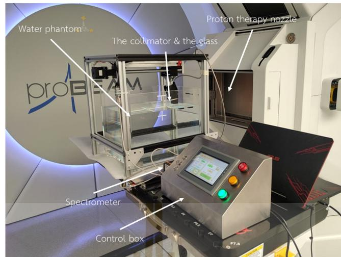
**Figure 5.6** The setup of the water phantom of the depth-dose profile at KCMH.
