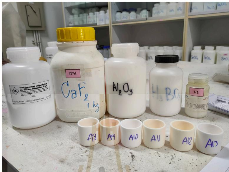
Figure A.1 Preparing and mixing the glass compositions in the alumina crucible.
