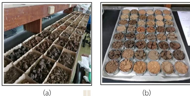
**Figure 4.1** Sample preparation before analysis in the laboratory. (a) a soil sample taken for air-dried; (b) a soil sample for moisture analysis taken in the oven.
