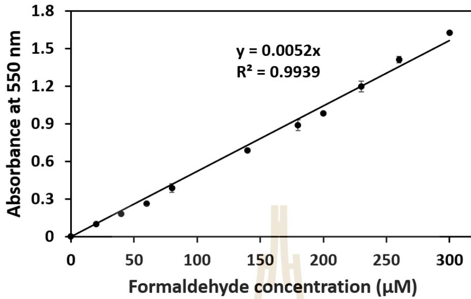
Figure 4.4 The calibration curve of formaldehyde standard solutions derivatized by the Purpald assay, in which absorption was recorded at 550 nm.
