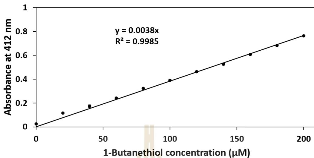
Figure 4.7 The calibration curve of 1-butanethiol standard solutions determined by the DTNB assay.
