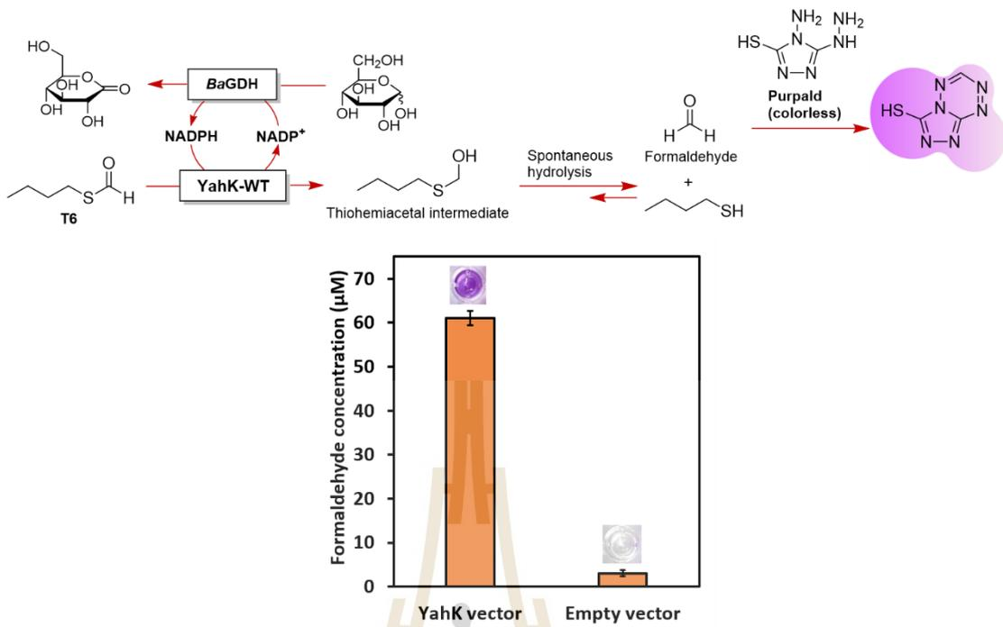
**Figure 4.9** Coenzyme regeneration tested by coupling *BaGDH* with the *YahK-WT* reaction. The reaction was performed by adding 500 µM T6, 10 µM NADP<sup>+</sup>, and 2 µM purified *BaGDH* into the lysate.
