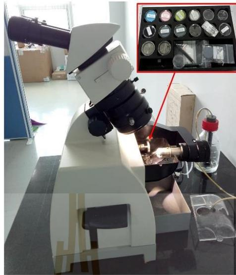
Figure 3.4 Target surfacing system (EM TMP, Leica, Germany).
