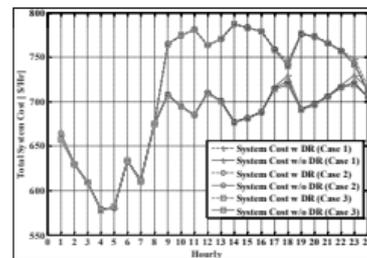
Fig. 6 Total System Cost with and without DR when Load Uncertainties represented by PTNF Sampling Methods
