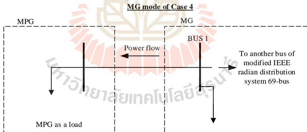
**Figure 4.6** Scenario 4 MG is supplying electric power
