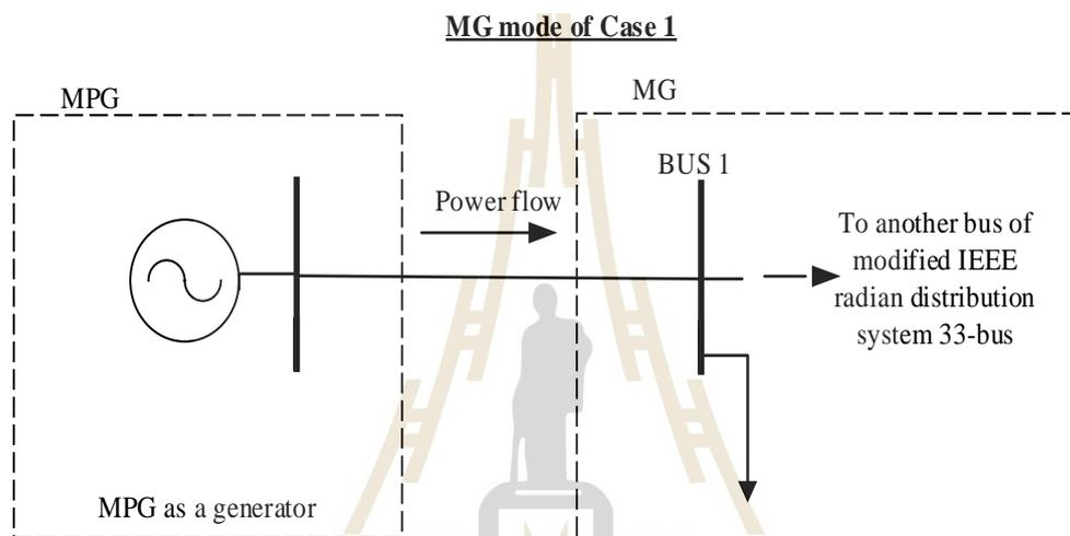
**Figure 4.2** Scenario 1 MG is receiving electric power
