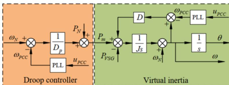
Figure 2.2 Active power controller of VGS
