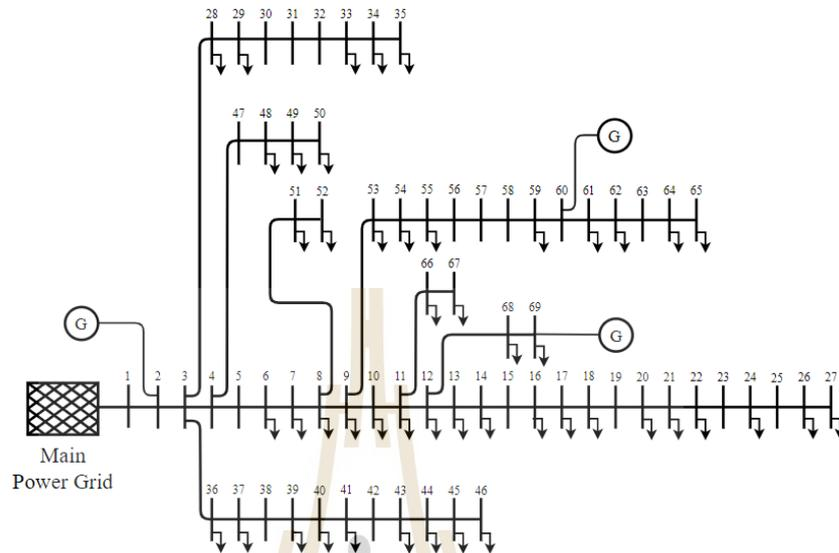
Figure B1.1 Modified IEEE radial distribution 69-bus system
