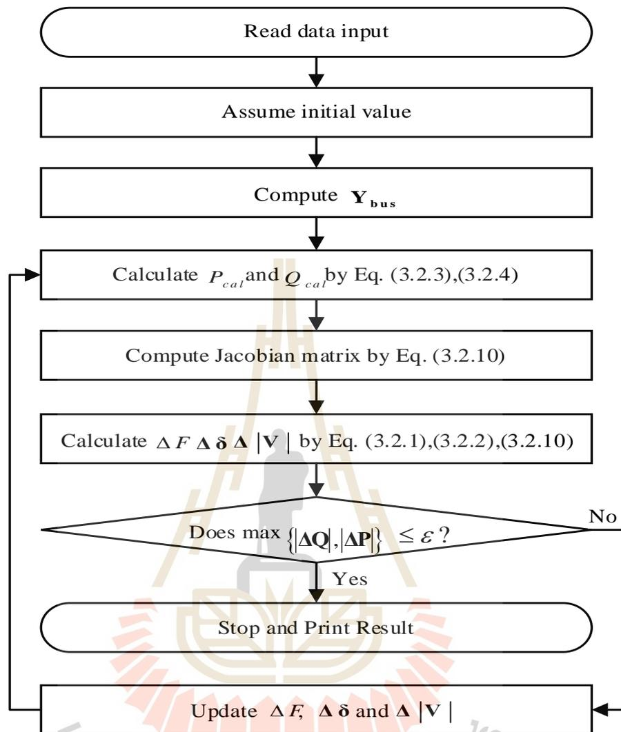
Figure 3.1 Computational procedure of power flow program for finding of the frequency deviation.
