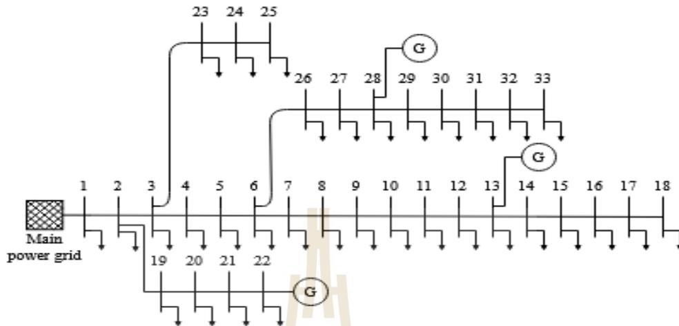
Figure A1.1 Modified IEEE radial distribution 33-bus system
