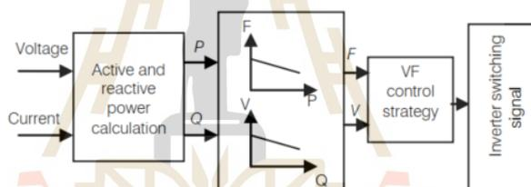
Figure 2.3 Droop based control system for the VF inverter
