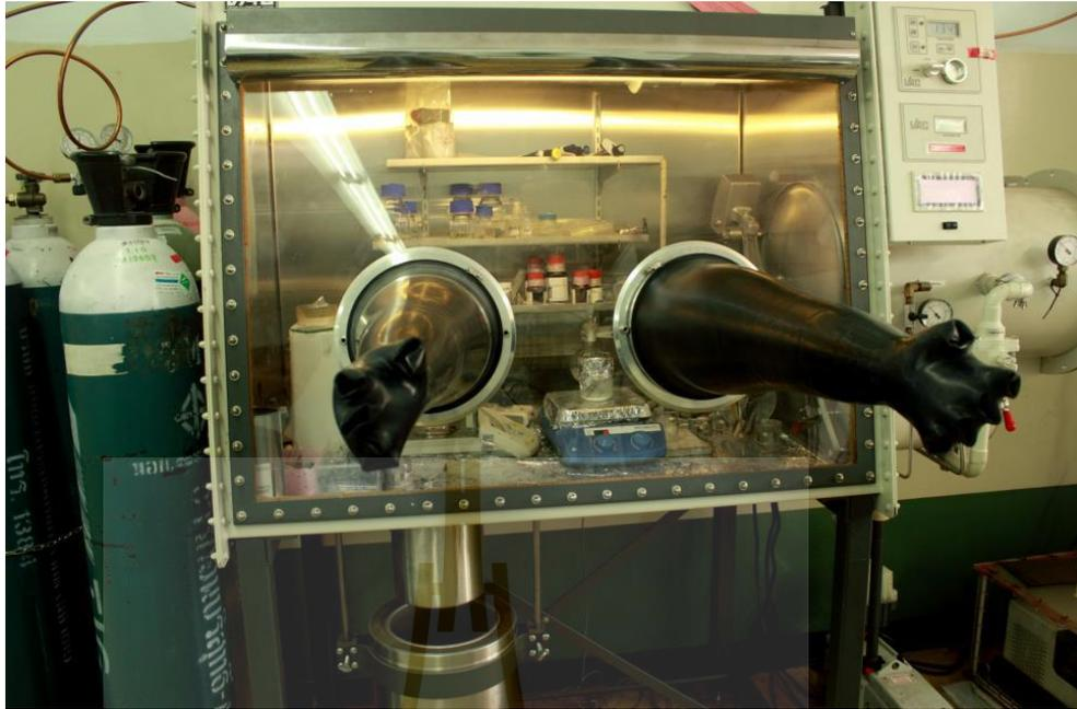
Figure 3.1 Glove box (Omni-Lab System, VAC) used in the laboratory.
