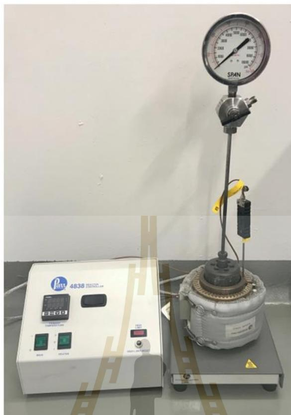
**Figure 3.3** Autoclave from Parr Instruments (4838 reactor controller).
