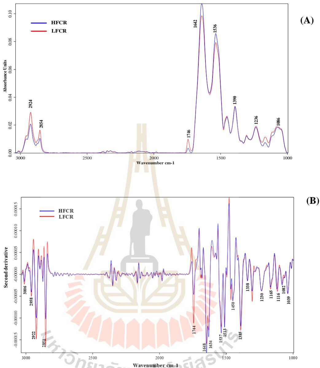
**Figure 4.1** (A) Average original spectra between high FCR and low FCR in thigh muscle. (B) 2nd derivative spectra between high FCR and low FCR. The IR spectra detected in spectra region from 4,000 to 400 cm<sup>-1</sup>, resolution 4 cm<sup>-1</sup>, with 64 scans.
