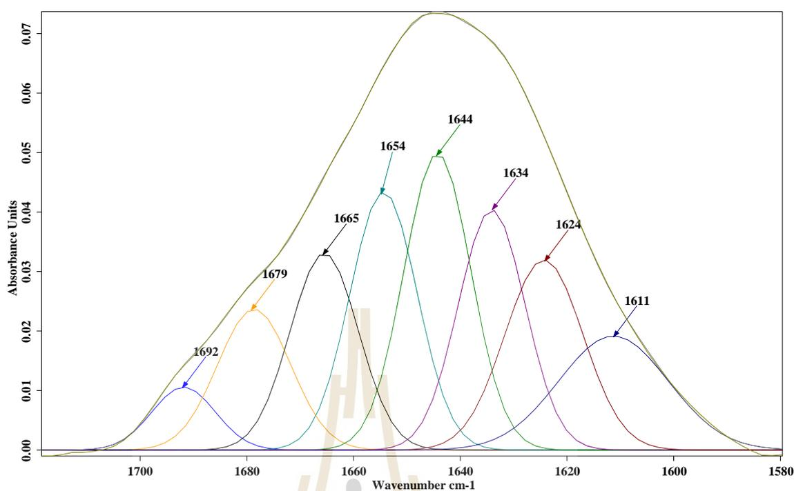
**Figure 4.4** The curve fitting of Amide I and secondary structure protein band assignment in thigh muscle by RFI.
