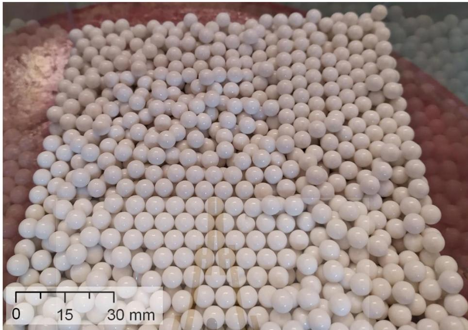
**Figure 3.1** ABS balls with uniform sizes of 6 mm used to simulate cavern roof and overburden.
