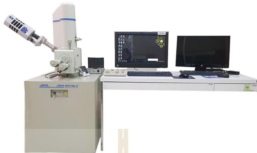
**Figure 4.18** JEOL JSM-6010LV scanning electron microscope used in this study.
