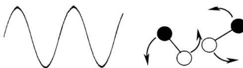
**Figure 2.3** Dipolar polarization mechanism.
