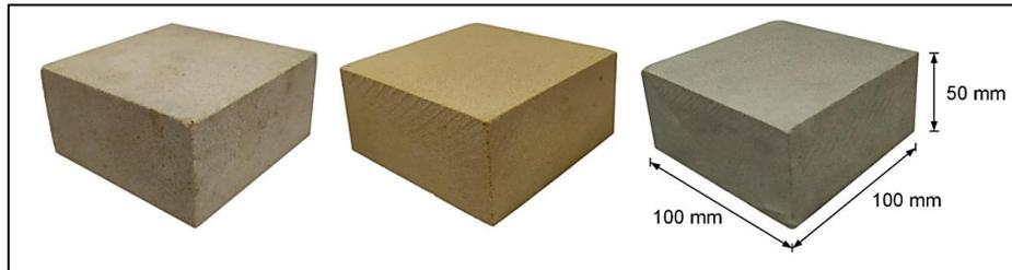
**Figure 3.1** Some rectangular block specimens of Phra Wihan, Phu Phan and Phu Kradung sandstones used in CERCHAR test on saw-cut surface.
