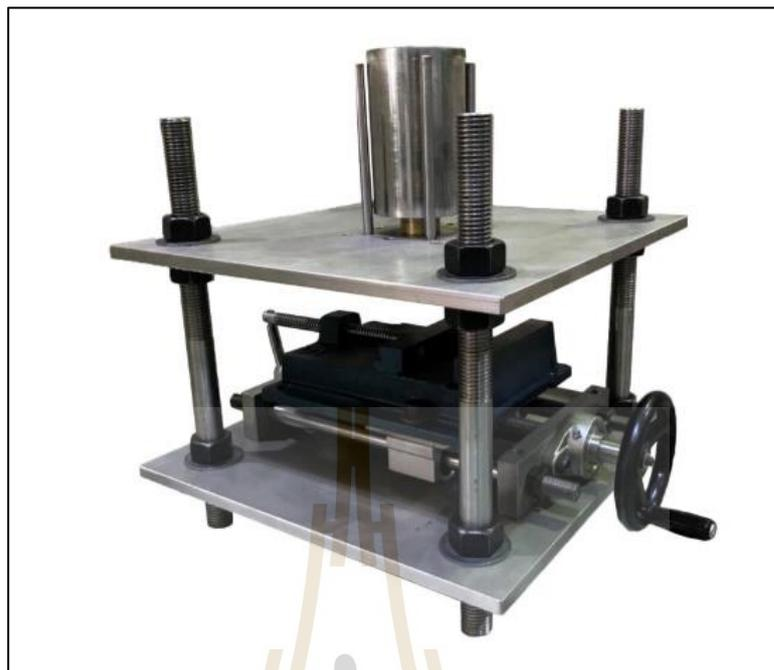
**Figure 1.2** Test equipment similar to West apparatus.
