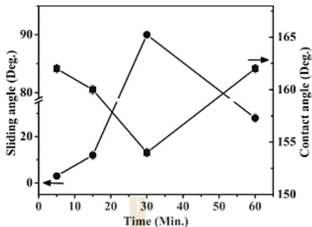
**Figure 2.6** Water contact angle and sliding angle on CuO surface in difference immerse time. (Li, Liu, Ye, Zhou, and Chen, 2011).
