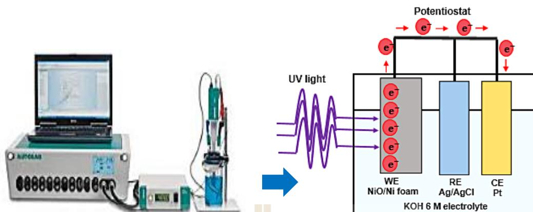
**Figure 3.5** Cyclic voltammetry measurement setup.
