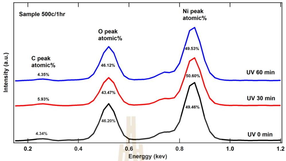
**Figure 4.8** EDS of Ni foam as the effect of UV light for Ni foam 500 °C/1hr.
