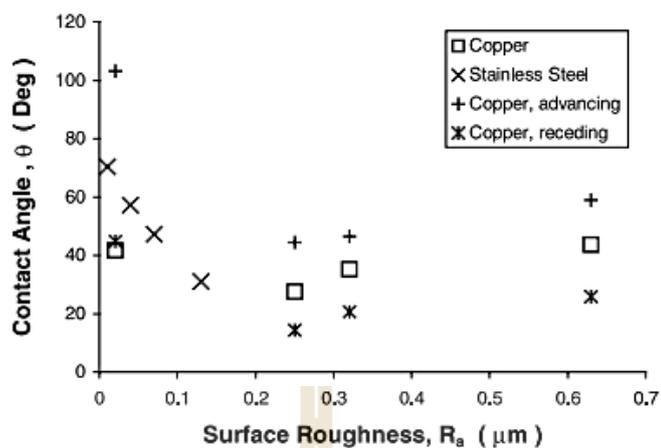
**Figure 2.7** Equilibrium contact angle versus surface roughness for copper and stainless steel surface. (Kandlikar and Steinke, 2002)
