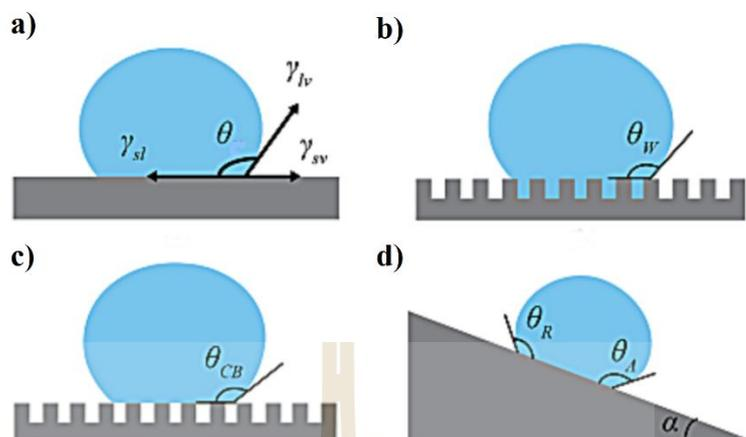
**Figure 2.3** The model of liquid droplet (a) Young's model, (b) Wenzel's model, (c) Cassie-Baxter's model, (d) liquid droplet on an incline showing advancing and receding contact angle and sliding angle (Tam, Palumbo, and Erb, 2016).
