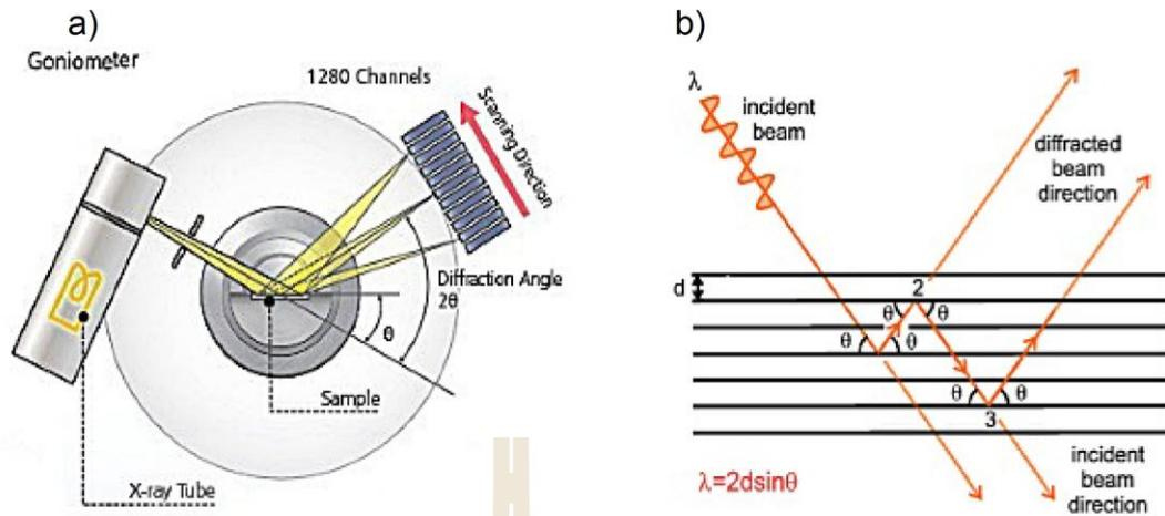
**Figure 3.2** The x-ray diffraction principle (a) inside the instrument and (b) procedure of x-ray diffraction process.
