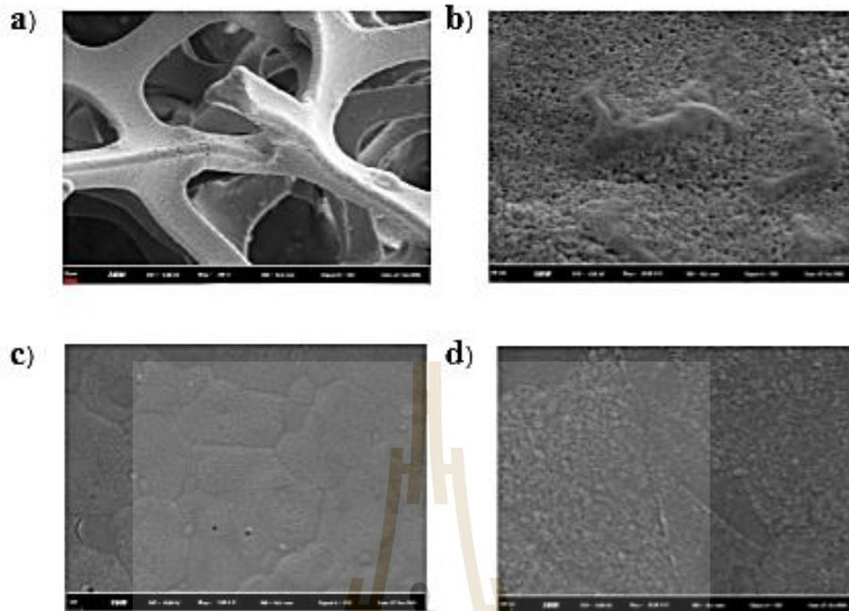
**Figure 4.3** SEM images of NiO/Ni foam annealed at 400 °C (a) for 1 hr, (b) magnification of (a), (c) annealed for 2 hr, and (d) magnification of (c).
