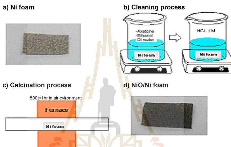
**Figure 3.1** The sample preparation process (a) Ni foam before cleaning, (b) Ni foam in cleaning process, (c) calcination process, and (d) NiO/Ni foam.
