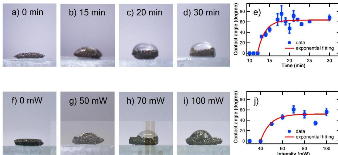
**Figure 4.10** Droplet Photographs and contact angle measured in two different conditions (a-e) the different exposure time with fixed intensity (50 mW) and (f-j) the different intensity with fixed time (30 min).
