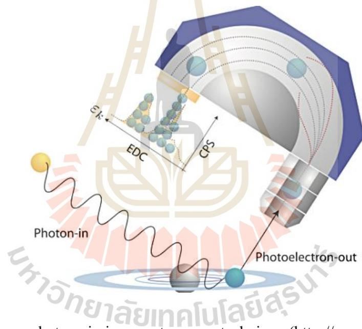
**Figure 3.6** X-ray photoemission spectroscopy technique (<http://www.slri.or.th>).
