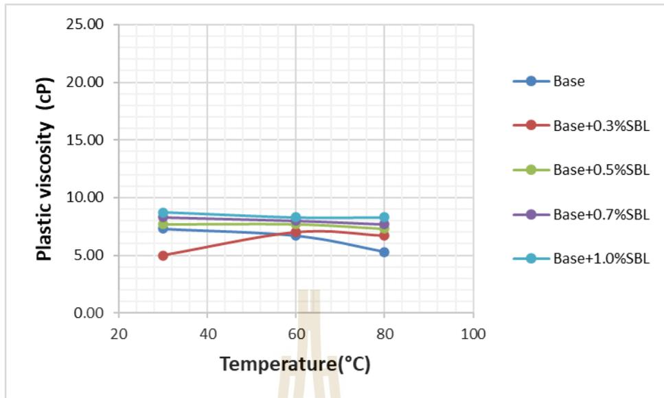
**Figure 4.10** Plastic viscosity of drilling mud mixed with various SBL versus temperature.
