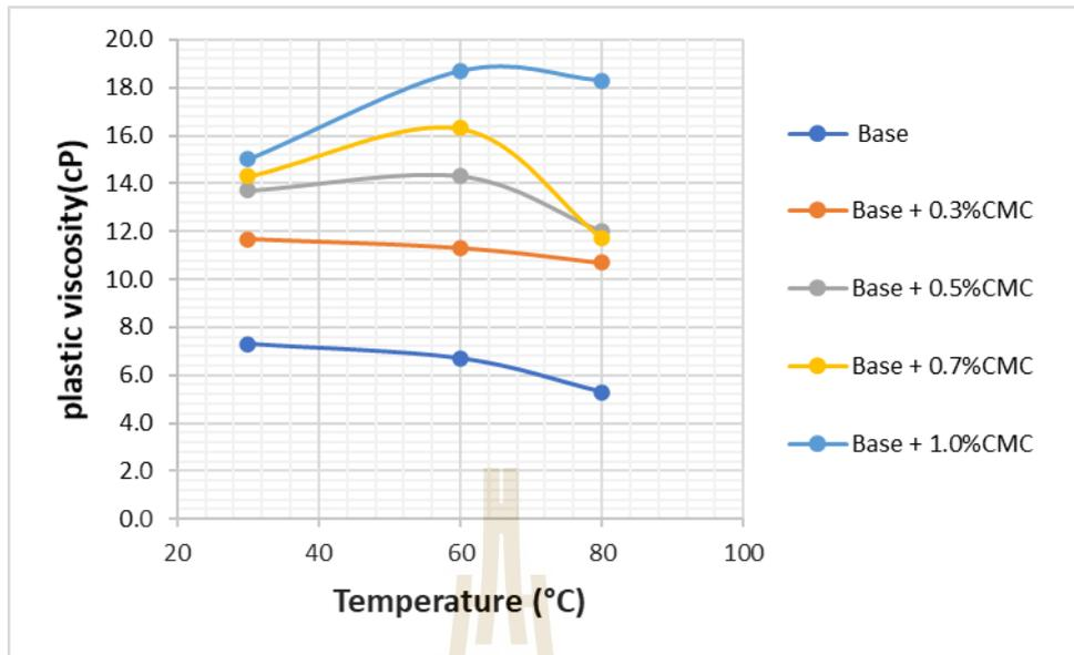
**Figure 4.12** Plastic viscosity of drilling mud mixed with various CMC versus temperature.
