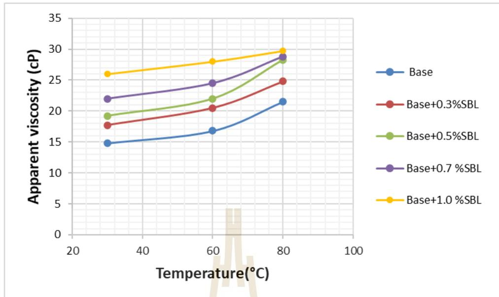
**Figure 4.6** Apparent viscosity of drilling mud mixed with various SBL versus temperature.
