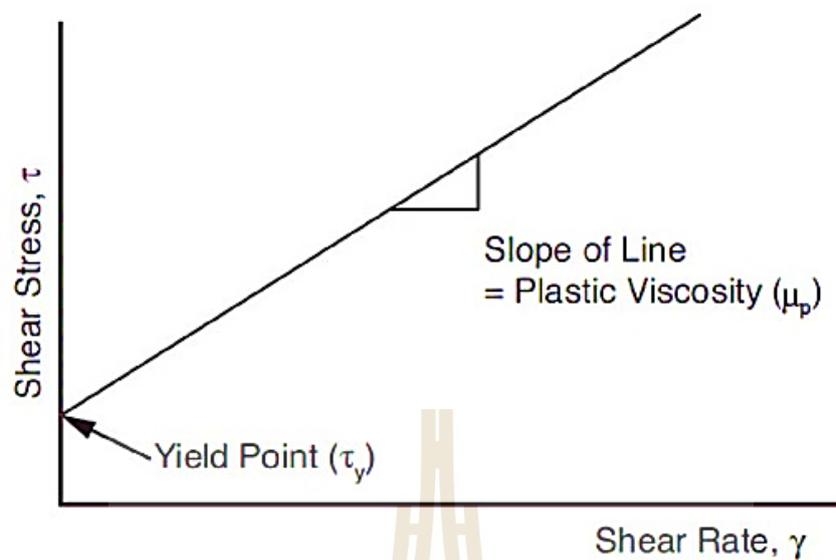
**Figure 2.1** Flow curve for the Bingham plastic model
