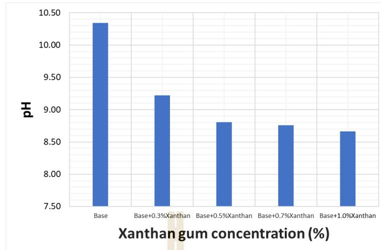
**Figure 4.32** The pH of drilling mud mixed with various concentrations of Xanthan gum at 30°C.
