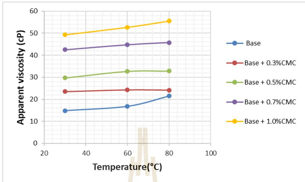
**Figure 4.8** Apparent viscosity of drilling mud mixed with various CMC versus temperature.
