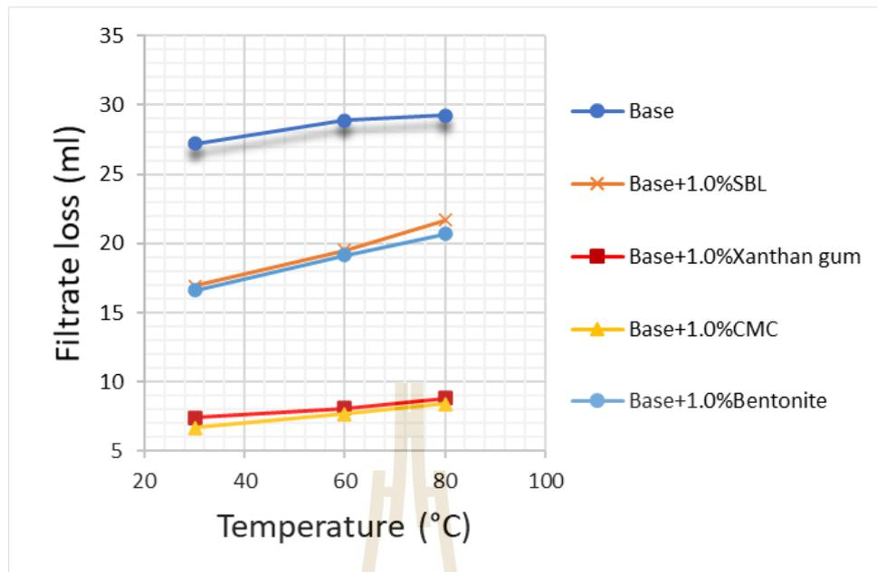
**Figure 4.29** API filtrate loss of drilling mud mixed with 1.0% of SBL, Xanthan gum, CMC, and Bentonite versus temperature at 30 minutes.
