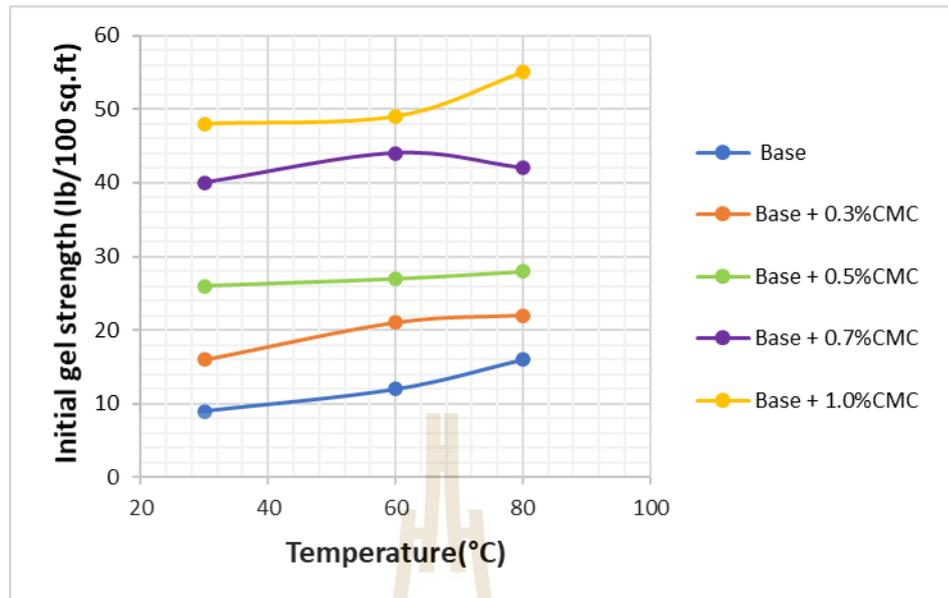
**Figure 4.20** Initial gel strength of drilling mud mixed with various CMC versus temperature.
