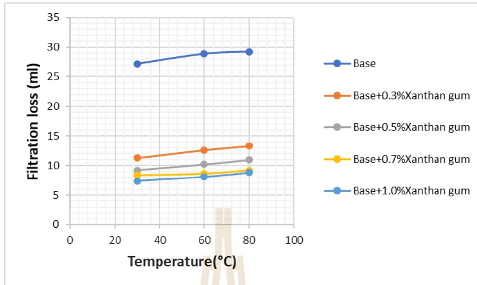
**Figure 4.27** API filtrated loss of drilling mud mixed with Xanthan gum concentration for 30 minutes versus temperature.
