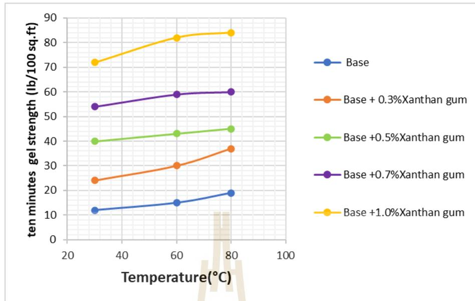
**Figure 4.22** Ten minutes gel strength of drilling mud mixed with various Xanthan gum versus temperature.
