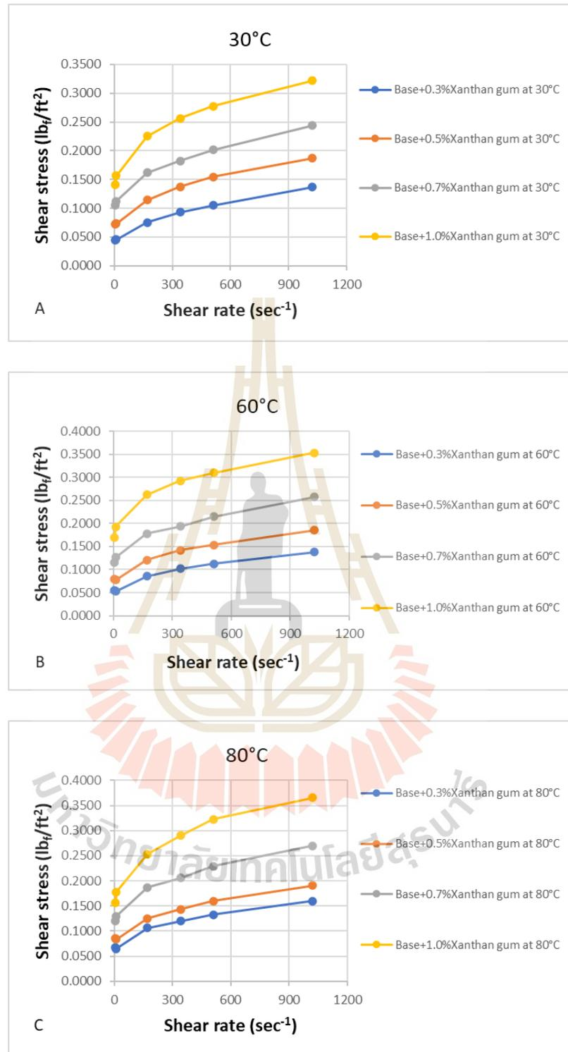
**Figure 4.4** rheological test of drilling mud mixed with 0.3, 0.5, 0.7, and 1.0% Xanthan gum under 30°C (A), 60°C (B), and 80°C (C).
