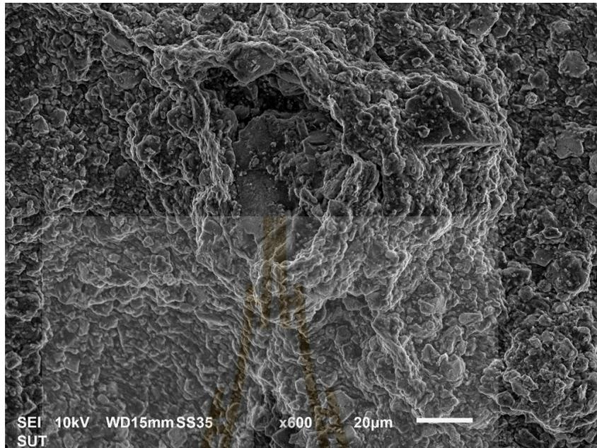
**Figure A1** The Characteristics of the surface of drilling mud mixed with SBL
