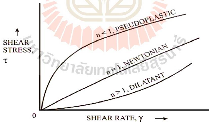
**Figure 2.2** Flow curve for the Power-law model.
