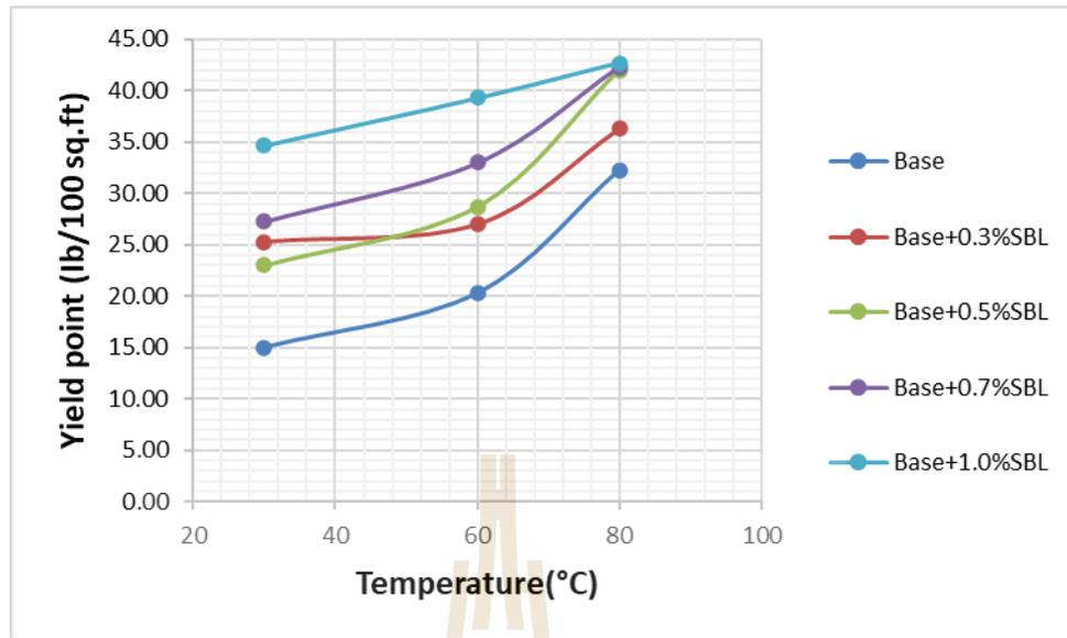
**Figure 4.14** Yield point of drilling mud mixed with various SBL versus temperature.
