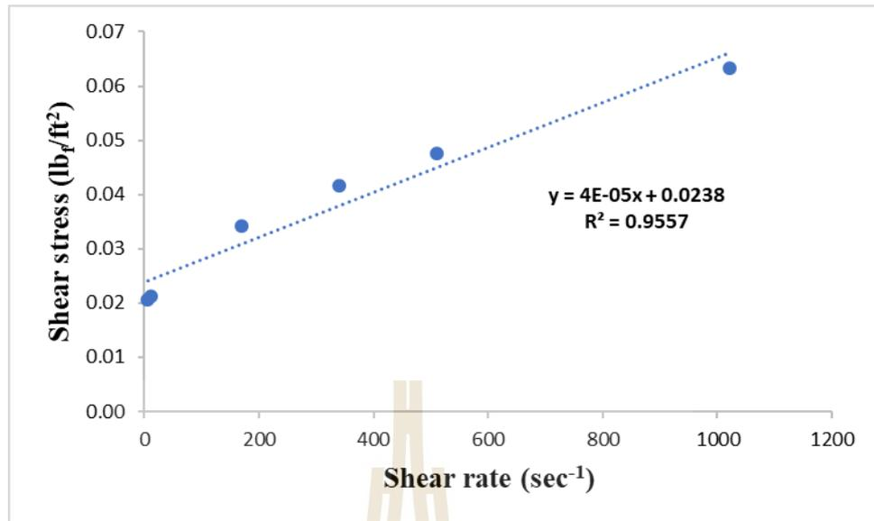
**Figure 4.1** Consistency plot of base bentonite mud at 30°C with a linear correlation.
