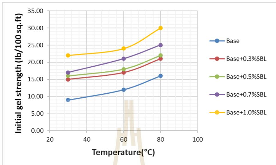
**Figure 4.18** Initial gel strength of drilling mud mixed with various SBL versus temperature.
