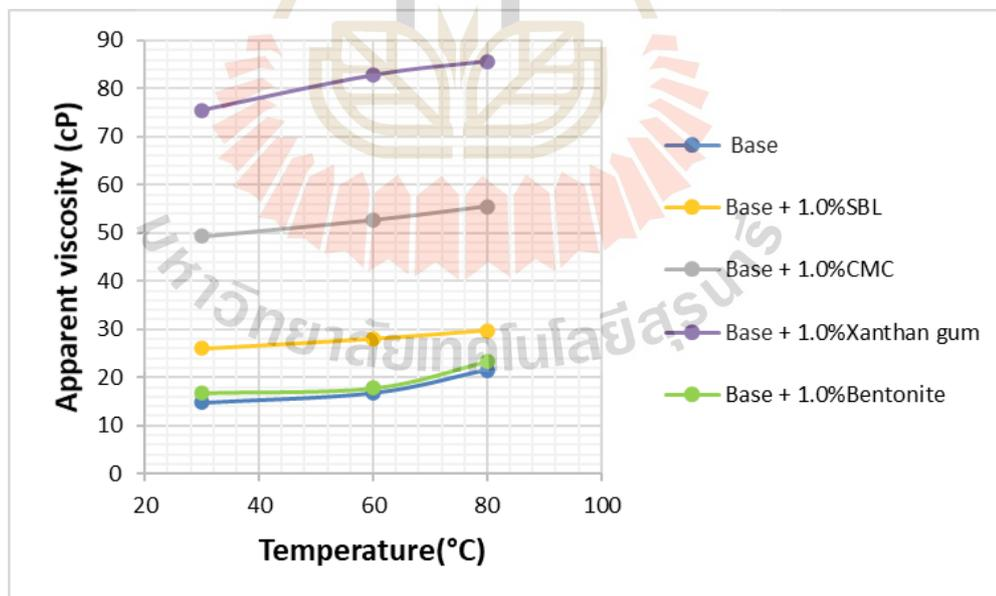
**Figure 4.9** Apparent viscosity of drilling mud mixed with 1.0% of SBL, Xanthan gum, and CMC versus temperature.
