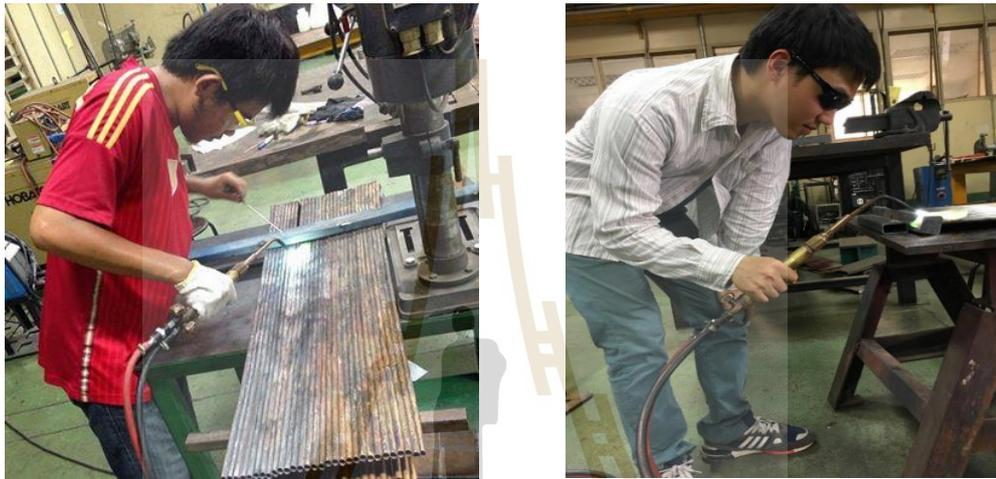
**Figure 3.2** Welding copper tubes
