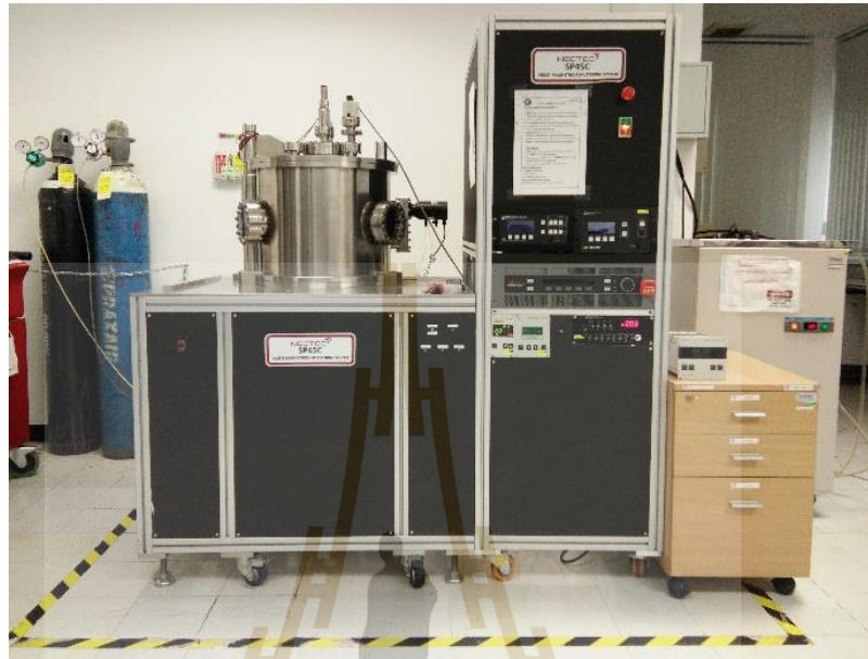
Figure 3.1 The pulsed DC magnetron sputtering system by OEC laboratory.
