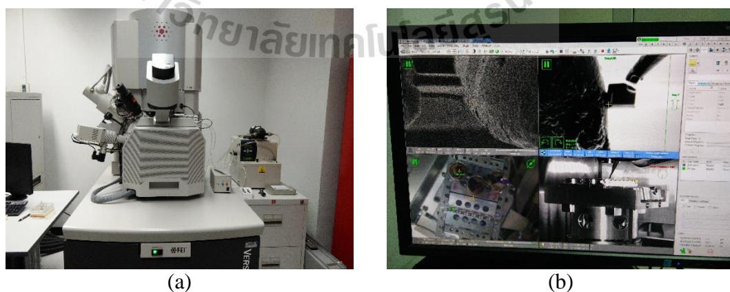
Figure 3.9 (a) FIB at NANOTEC and (b) monitors for prepare samples.
