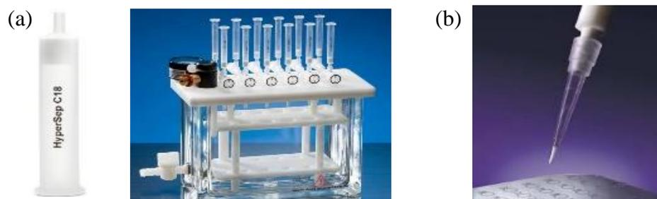
**Figure 1.12** (a) SPE cartridges with a chamber and a vacuum pump (b) a commercial micro-pipette tip SPE.
