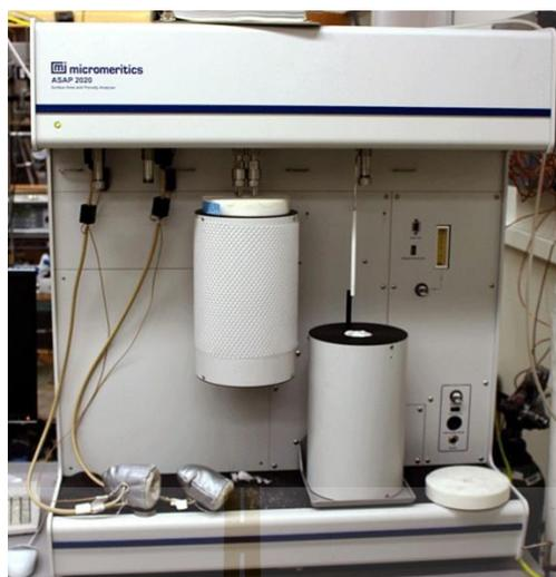
**Figure 3.20** The Micromeritics ASAP 2020 plus.
