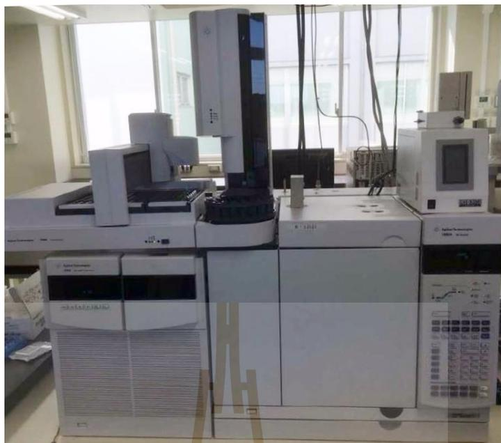
**Figure 3.12** The Agilent 7000B GC/MS
