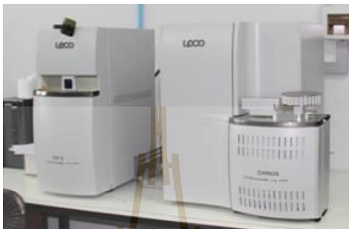
**Figure 3.14** Carbon, Hydrogen and Nitrogen (CHN) determinator series 628 LECO.
