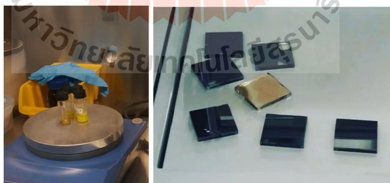
Figure 2.7 The precursor for prepared  $\text{CH}_3\text{NH}_3\text{PbI}_3$ ,  $\text{CH}_3\text{NH}_3\text{PbI}_{(3-x)}\text{Cl}_x$ . And film after annealing.
