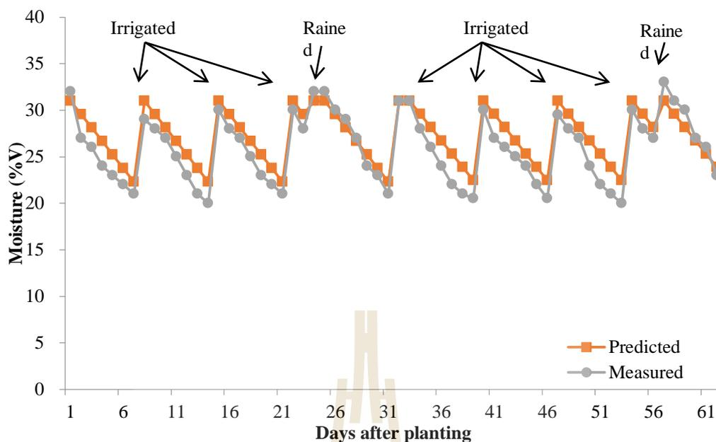
**Fig 3.4** Predicted and measured soil moisture content during the 3<sup>rd</sup> and 4<sup>th</sup> MAP in SCL soil.
