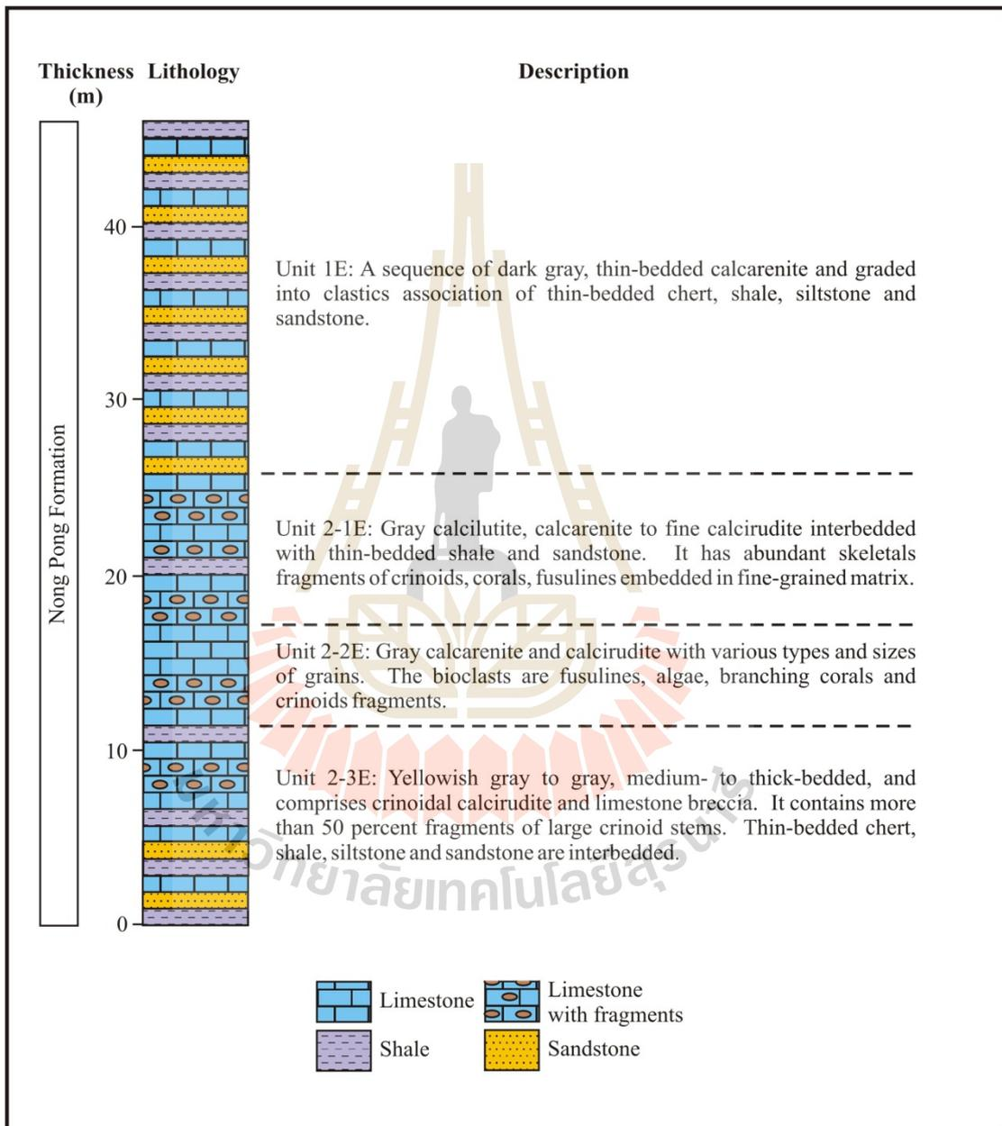
**Figure 4.19** The lithostratigraphic column of the Old quarry.
