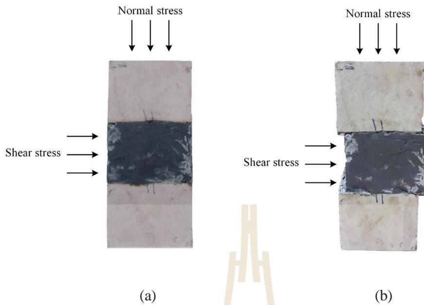
**Figure 5.11** Some specimen of grouting material in sandstone rock fracture before (a) and after (b) failure under shearing.
