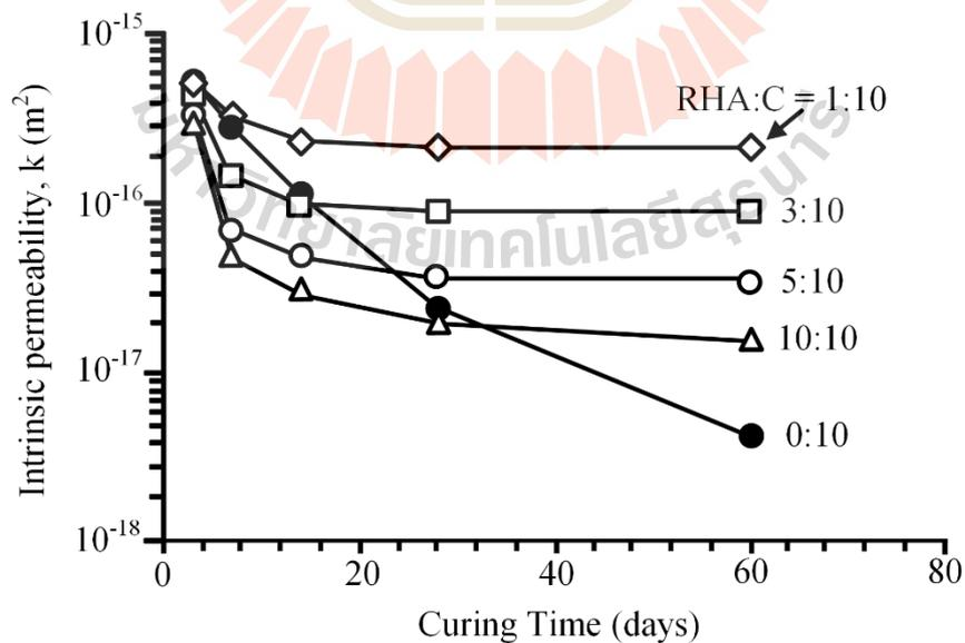
**Figure 6.3** Intrinsic permeability as a function of curing time.
