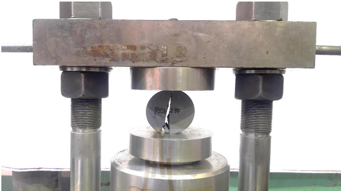
**Figure 5.7** Brazilian tensile strength test with constant loading rate.
