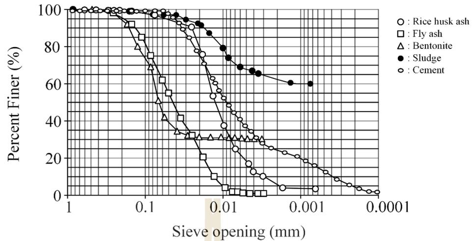
**Figure 3.2** The particle size distribution of rice husk ash compared with those of fly ash, sludge, bentonite and cement results (Chiangmai, 2016 and Wetchasat, 2013).
