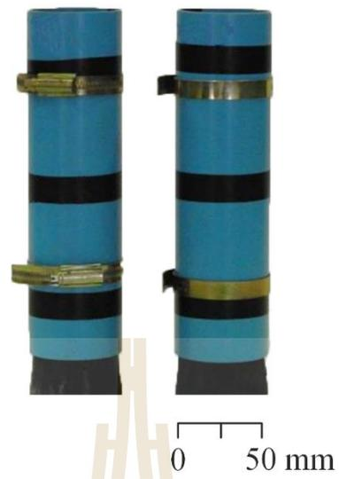
**Figure 3.4** PVC molds with curing cement mixture.
