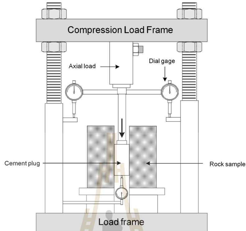
**Figure 5.18** Schematic drawing of push-out test.
