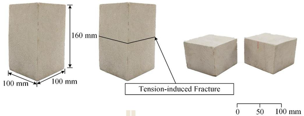
**Figure 3.6** Some sandstone samples are prepared for direct shear test.
