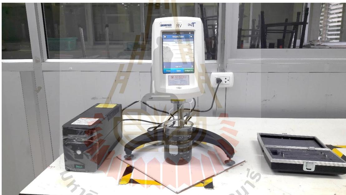
**Figure 4.6** The viscosity test of slurry measure by using the viscometer, Brookfield® viscometer DV2T 150 VA 50/60 Hz.
