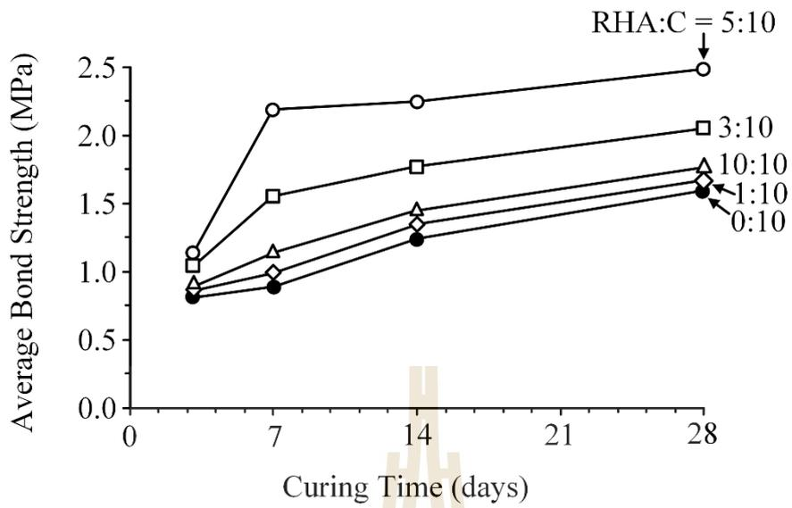
**Figure 5.20** Average bond strength as a function of curing time.
