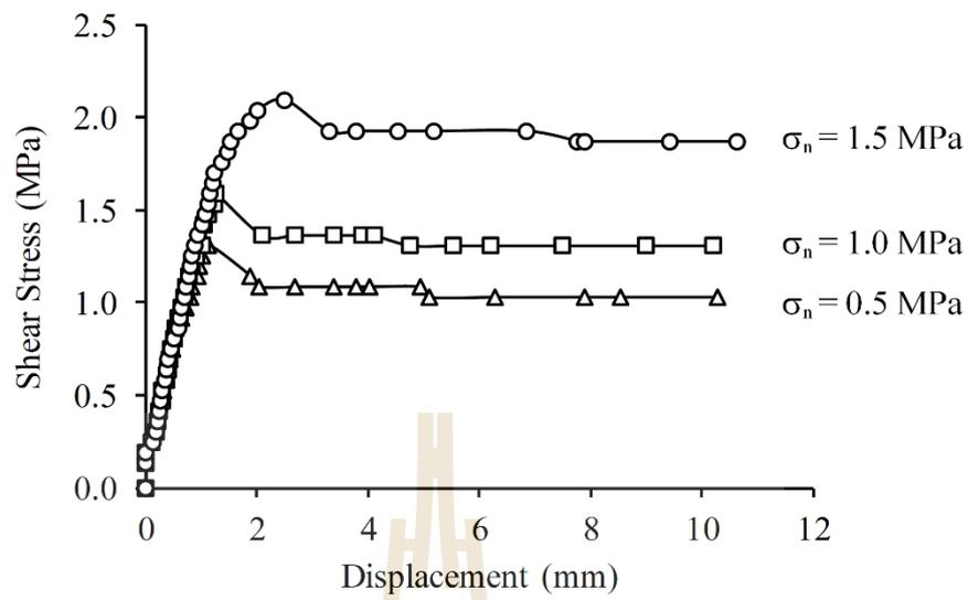
**Figure 5.16** Shear stress as a function of shear displacement for RHA:C = 10:10.
