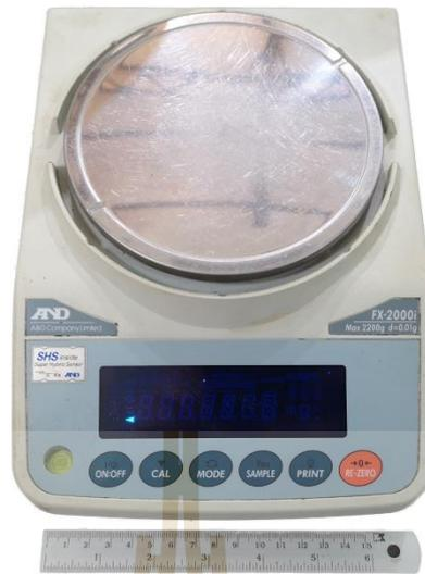
**Figure 4.3** Digital weight scale with maximum capacity of 2,200 g and accuracy to 0.01 g.
