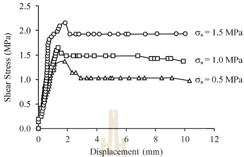
**Figure 5.14** Shear stress as a function of shear displacement for RHA:C = 3:10.
