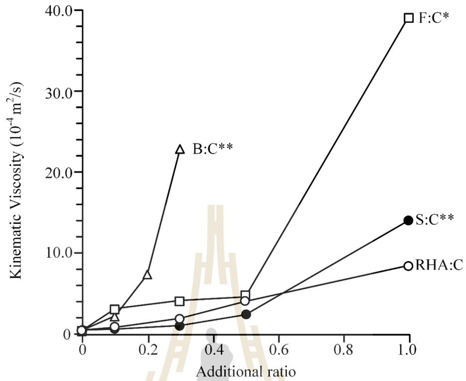
**Figure 4.7** Kinematic viscosity of mixture material for different ratios (\*Chiangmai, 2016 and \*\* Wetchasat, 2013).
