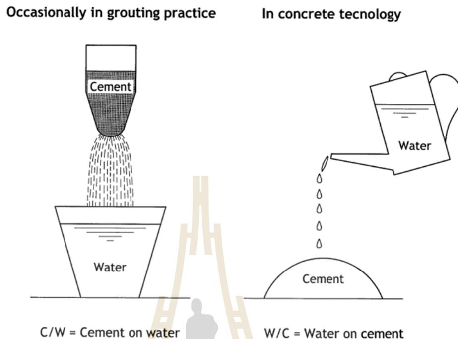
**Figure 2.1** Definition of the water to cement ratio (W/C) (Deere, 1982).
