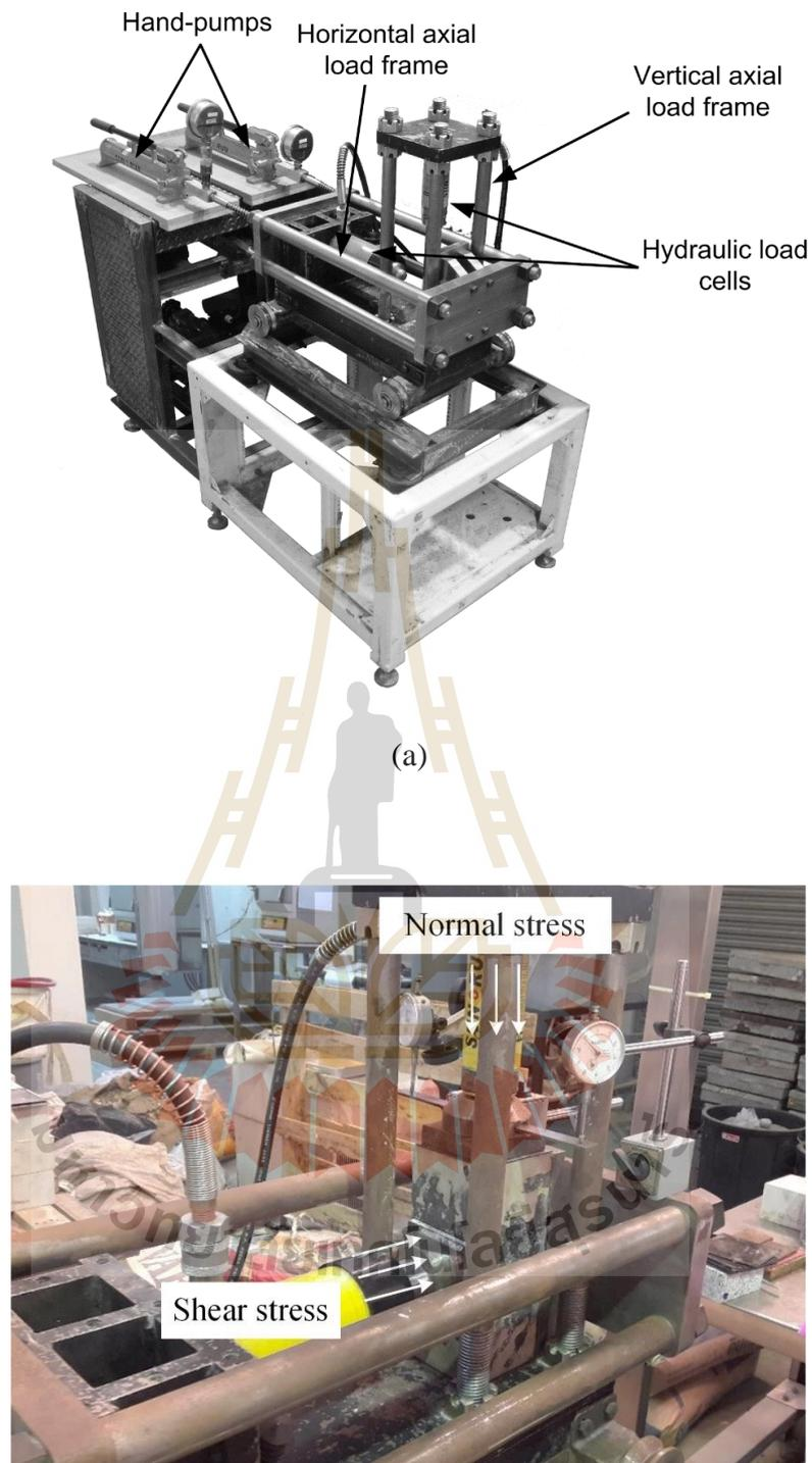
**Figure 5.10** Laboratory arrangement for direct shear test (Boonyord, 2017) (a) and during testing (b).
