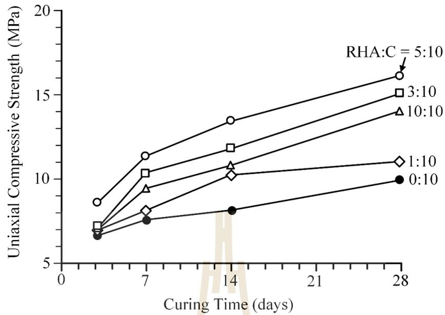
**Figure 5.4** Uniaxial compressive strengths of grouting materials as a function of curing time.
