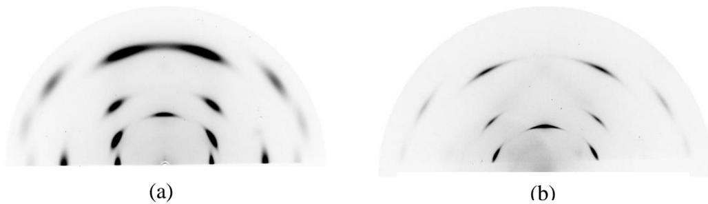
**Figure 4.8** 2D GIXRD diffraction images of AZO dense films with fixed grazing angle of (a)  $0.5^\circ$  and (b)  $10^\circ$
