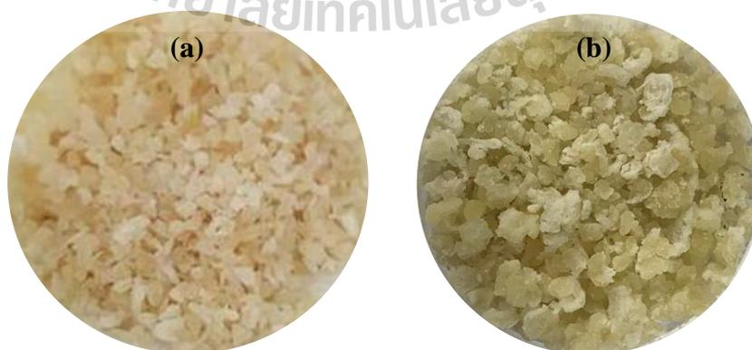
**Figure 4.10** Fresh (a) and used (b) aluminum alginate catalyst
