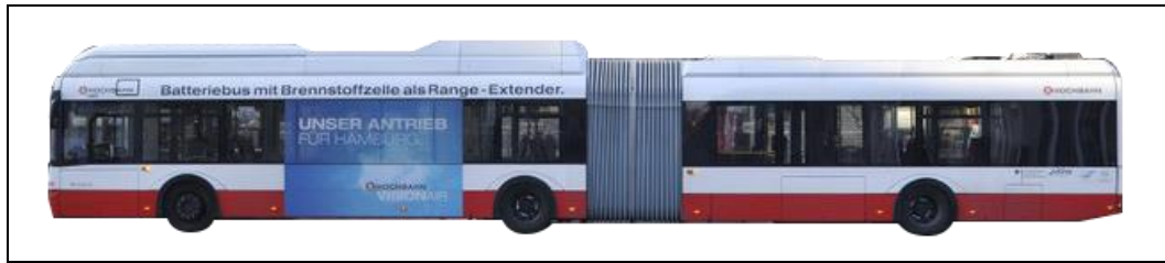
Figure 3.6 The first 18 m long pure electric articulated bus
