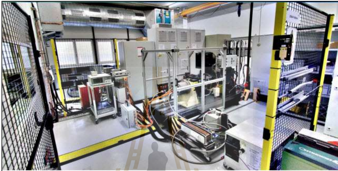
Figure 4.1 DRIVETEK AG test bench of traction motor
