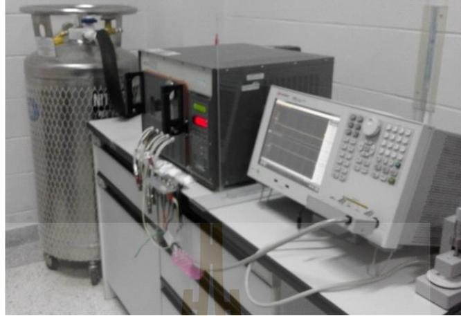
**Figure 3.12** Shows Agilent 4294A precision impedance analyser, KKKU.
