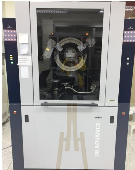
**Figure 3.8** Shows X-ray diffraction machine, D8-Bruker, SUT.
