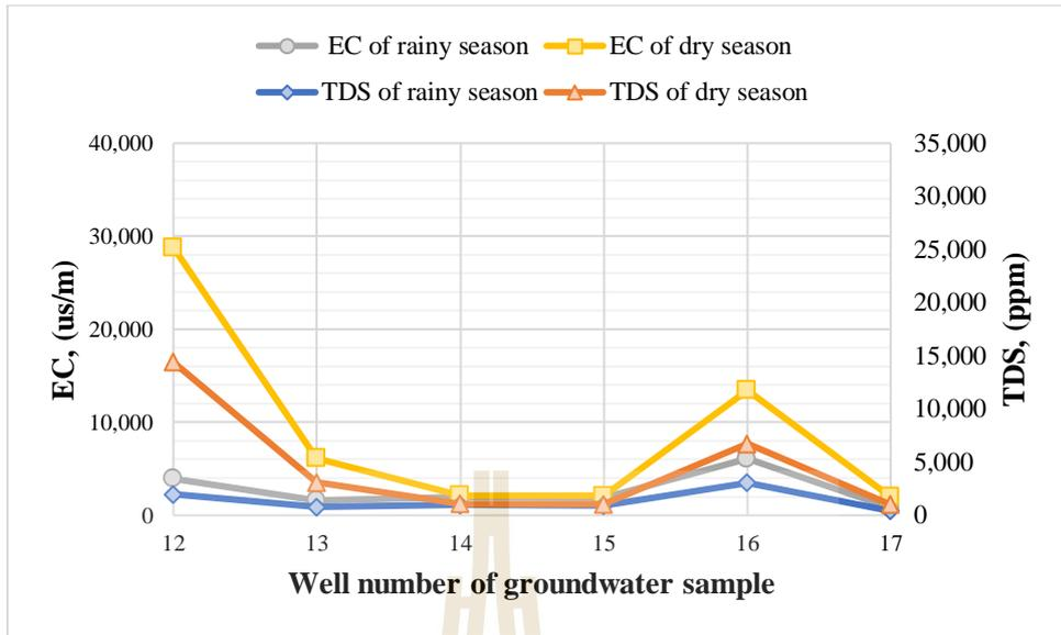
**Figure 4.13** The electrical conductivity (EC) and total dissolved solids (TDS) of groundwater samples at Non Sung district.
