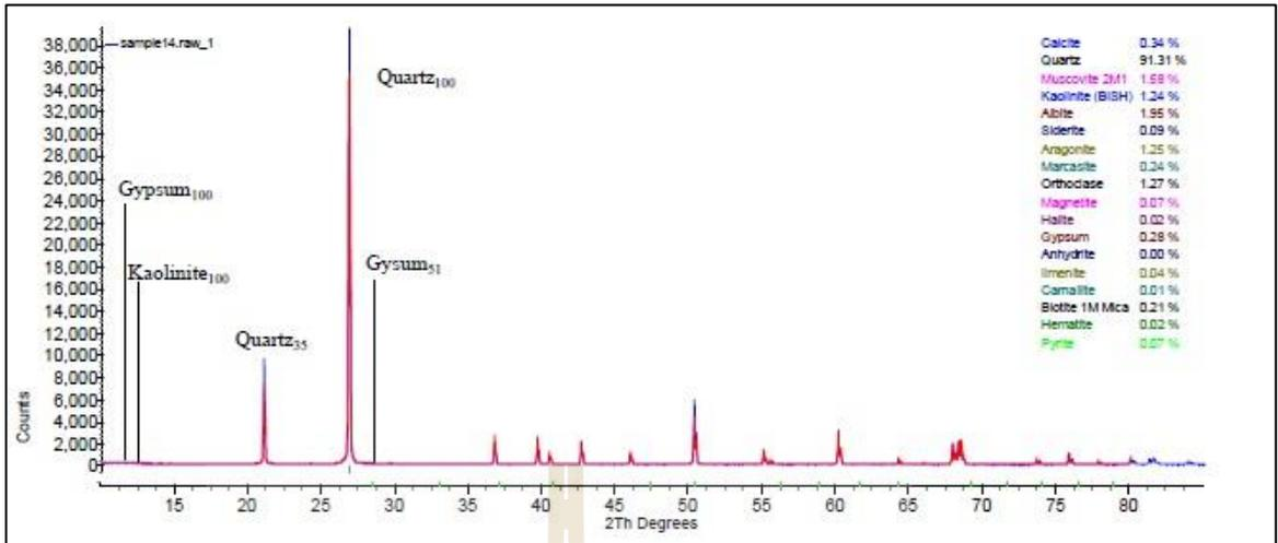
**Figure B.11** Interpretation of X-Ray Diffractometer analysis from site number 14.
