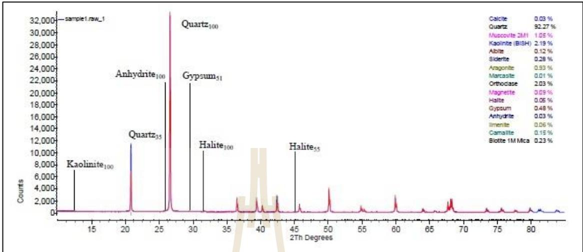
Figure B.1 Interpretation of X-Ray Diffractometer analysis from site number 1.
