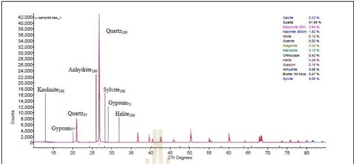
**Figure B.5** Interpretation of X-Ray Diffractometer analysis from site number 8.
