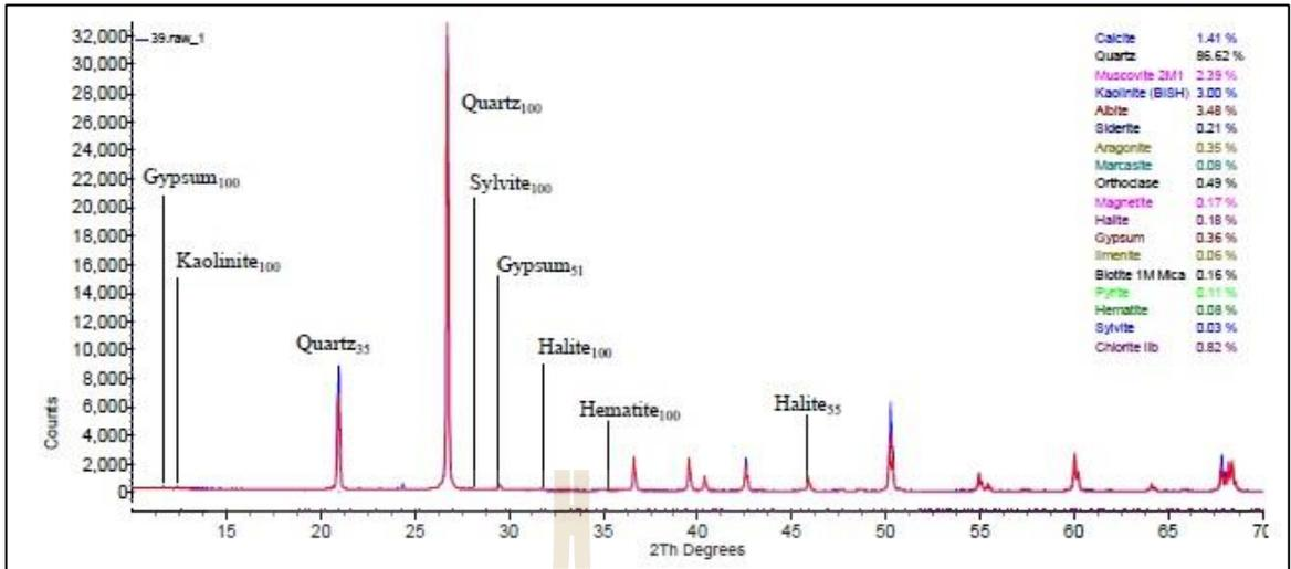
Figure B.33 Interpretation of X-Ray Diffractometer analysis from site number 39.
