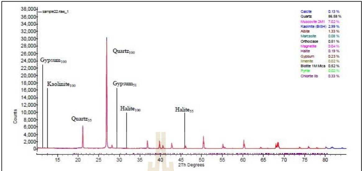
**Figure B.19** Interpretation of X-Ray Diffractometer analysis from site number 22.
