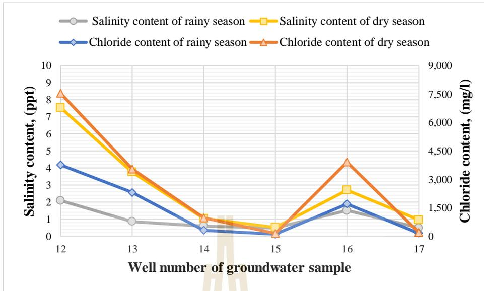
**Figure 4.24** The salinity content and chloride content of groundwater samples at Non Sung district.
