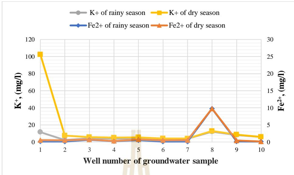
**Figure 4.44** Contents of potassium and iron ions of groundwater samples
