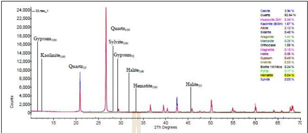
Figure B.29 Interpretation of X-Ray Diffractometer analysis from site number 33.
