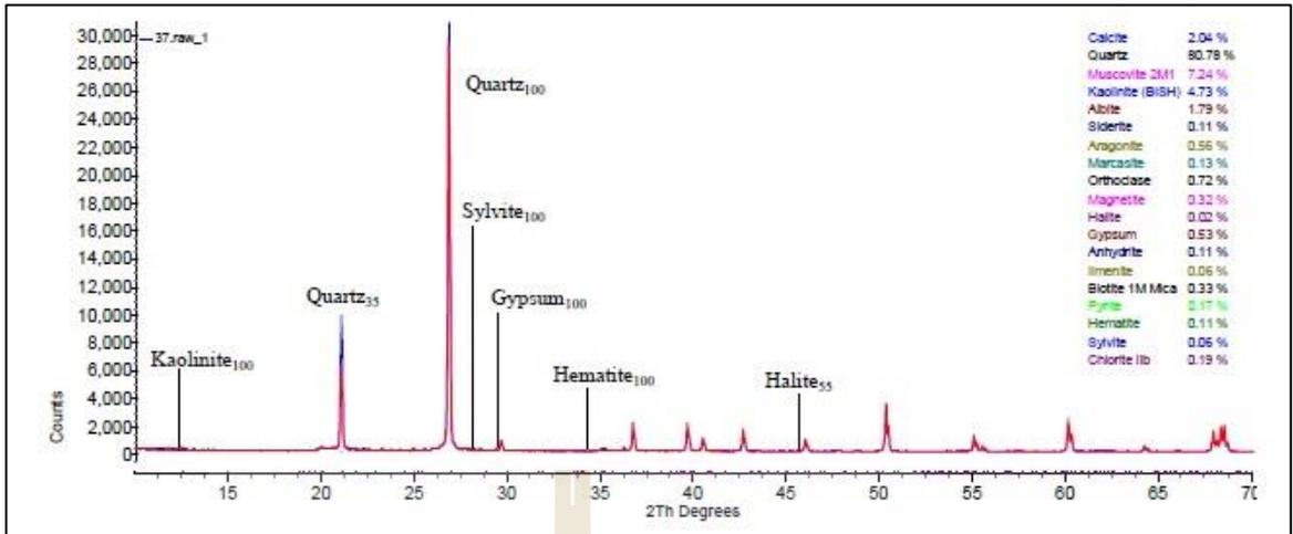
Figure B.31 Interpretation of X-Ray Diffractometer analysis from site number 37.
