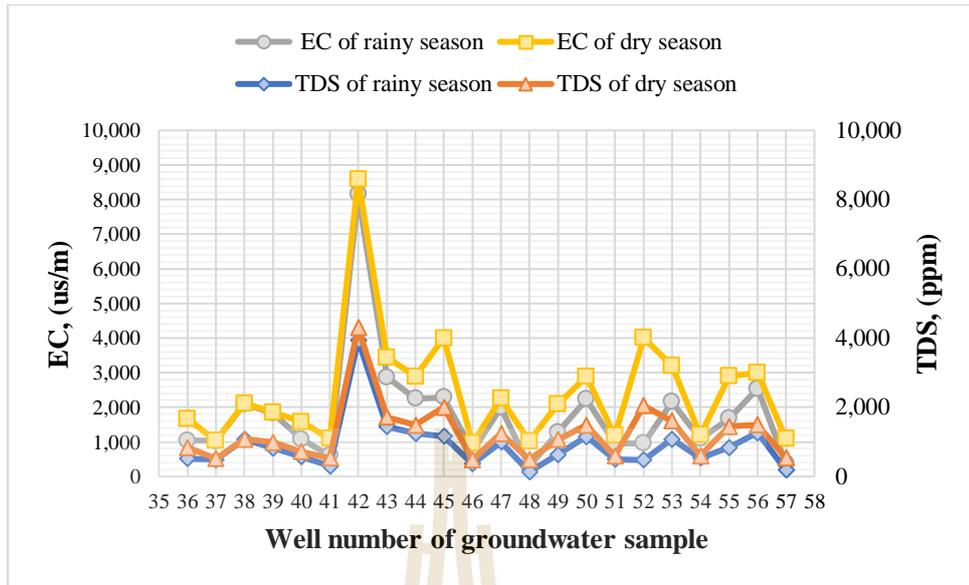
**Figure 4.15** The electrical conductivity (EC) and total dissolved solids (TDS) of groundwater samples at Kham Sakae Saeng district.
