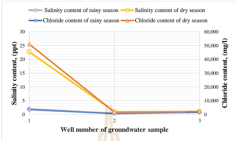
**Figure 4.22** The salinity content and chloride content of groundwater samples at Non Daeng district.
