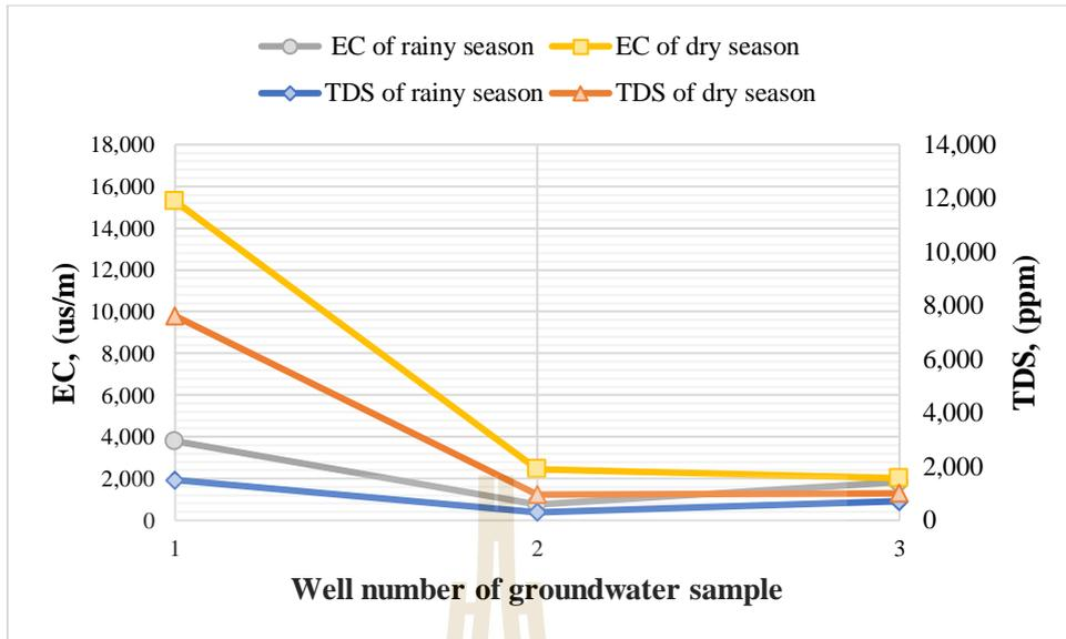
**Figure 4.11** The electrical conductivity (EC) and total dissolved solids (TDS) of groundwater samples at Non Daeng district.
