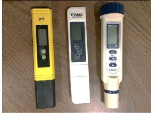
**Figure 3.5** The pH, electrical conductivity (EC) and total dissolved solids (TDS), and salinity content meters respectively from left to right.
