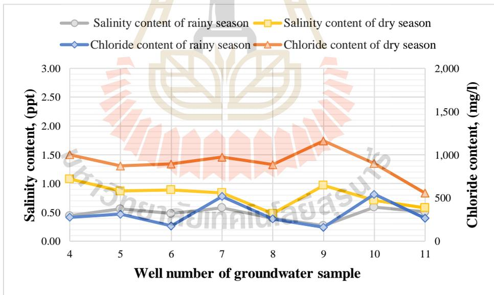
**Figure 4.23** The salinity content and chloride content of groundwater samples at Non Thai district.
