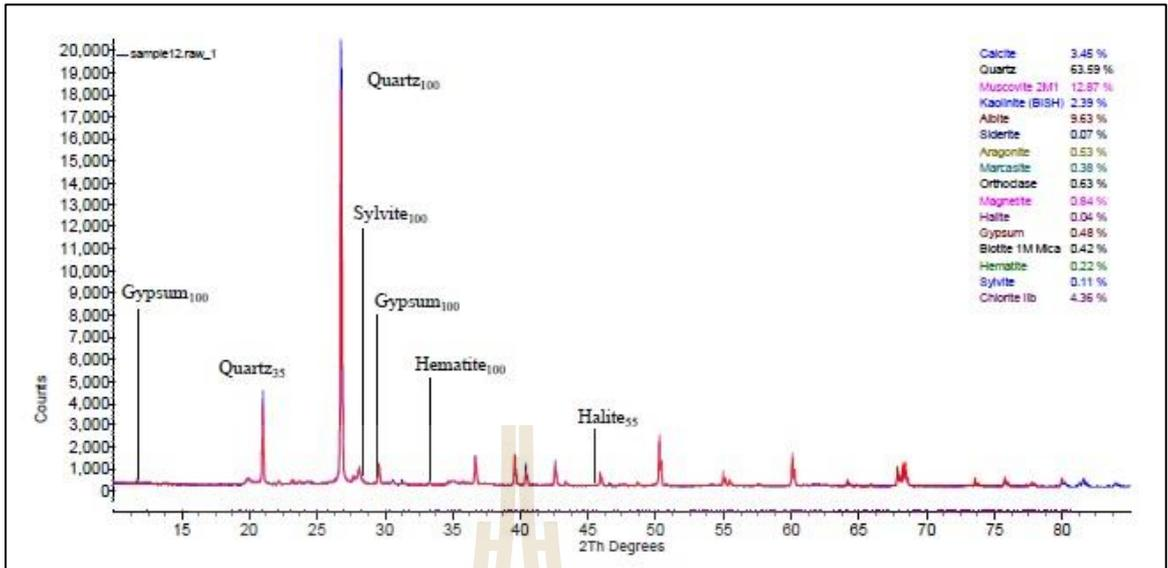
**Figure B.9** Interpretation of X-Ray Diffractometer analysis from site number 12.
