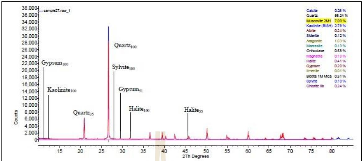
**Figure B.23** Interpretation of X-Ray Diffractometer analysis from site number 27.
