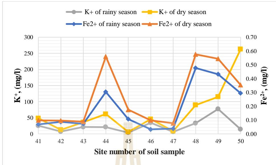
**Figure 4.41** Contents of potassium and iron ions of soil samples at Kham Sakae Saeng district.
