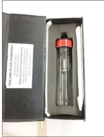
**Figure 3.10** Hollow cathode lamp.
