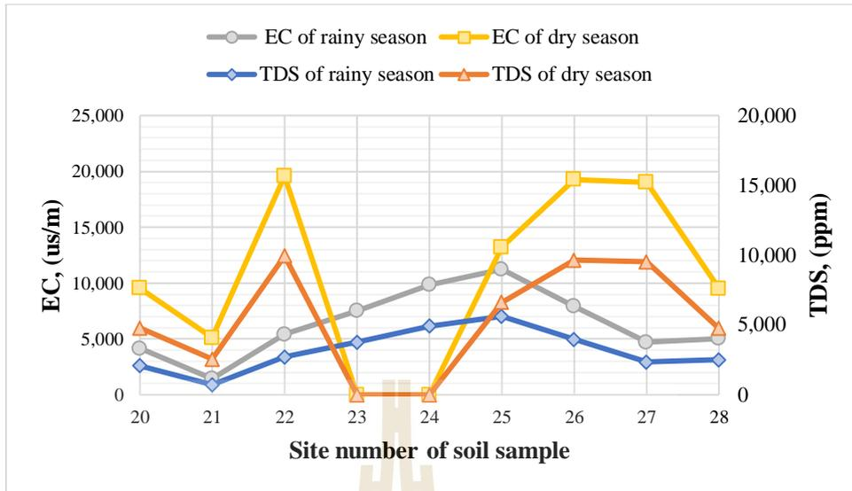
**Figure 4.8** The electrical conductivity (EC) and total dissolved solids (TDS) of soil samples at Non Sung district.
