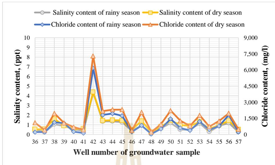
**Figure 4.26** The salinity content and chloride content of groundwater samples at Kham Sakae Saeng district.
