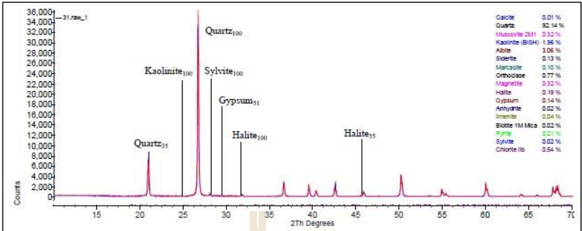
**Figure B.27** Interpretation of X-Ray Diffractometer analysis from site number 31.
