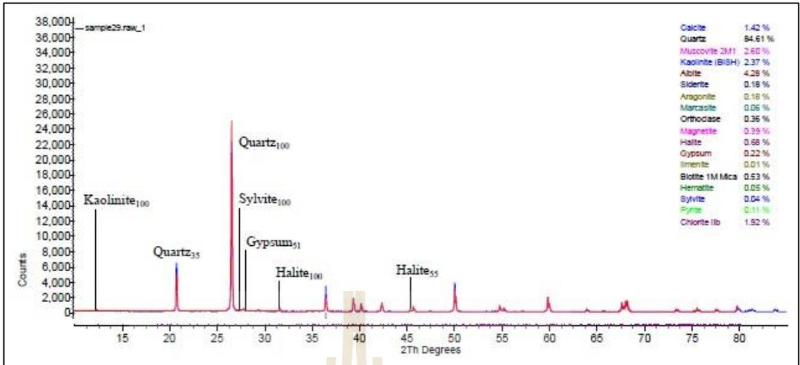
Figure B.25 Interpretation of X-Ray Diffractometer analysis from site number 29.
