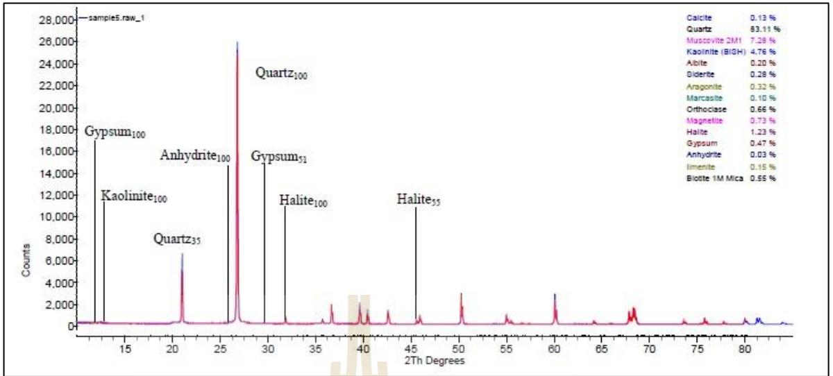
Figure B.3 Interpretation of X-Ray Diffractometer analysis from site number 5.
