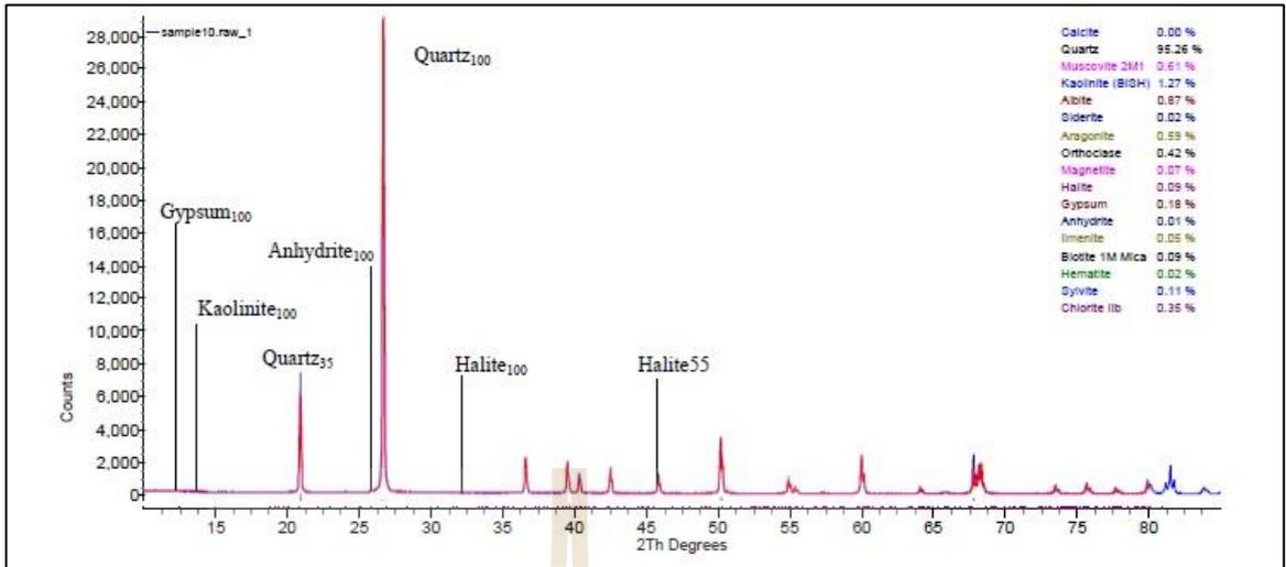
**Figure B.7** Interpretation of X-Ray Diffractometer analysis from site number 10.
