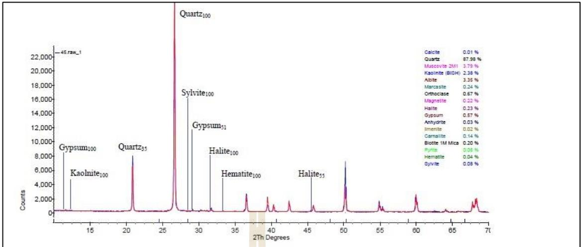
Figure B.35 Interpretation of X-Ray Diffractometer analysis from site number 45.
