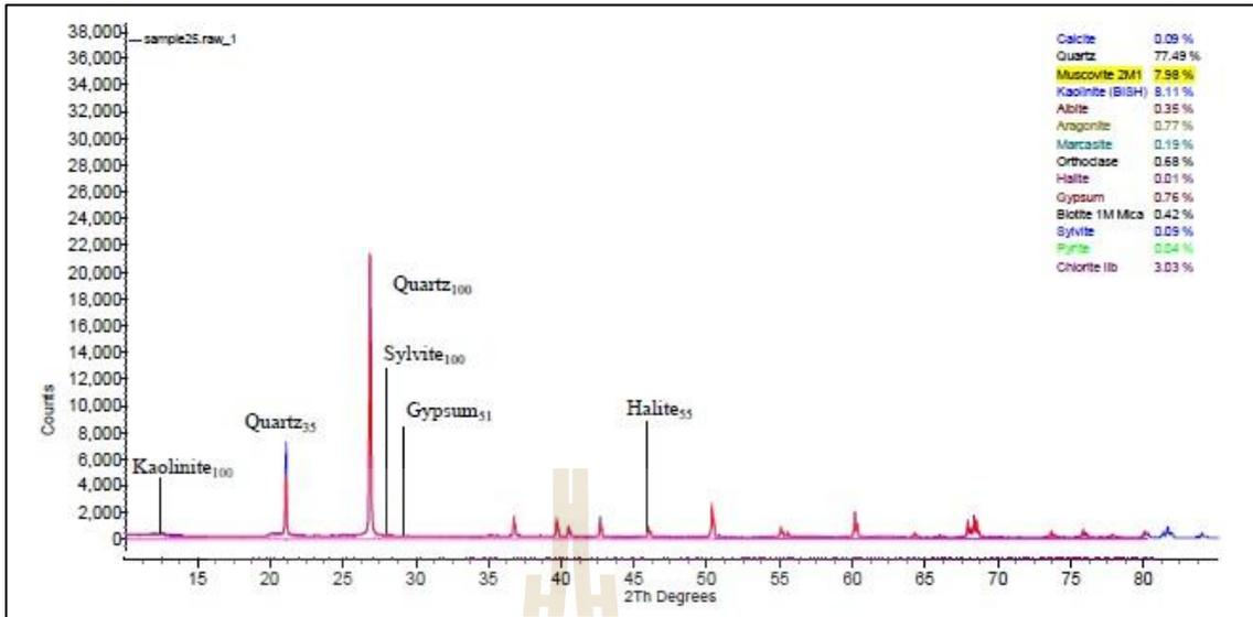
Figure B.21 Interpretation of X-Ray Diffractometer analysis from site number 25.
