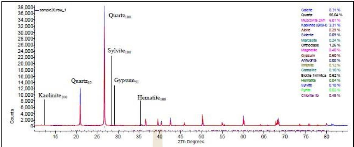
**Figure B.17** Interpretation of X-Ray Diffractometer analysis from site number 20.
