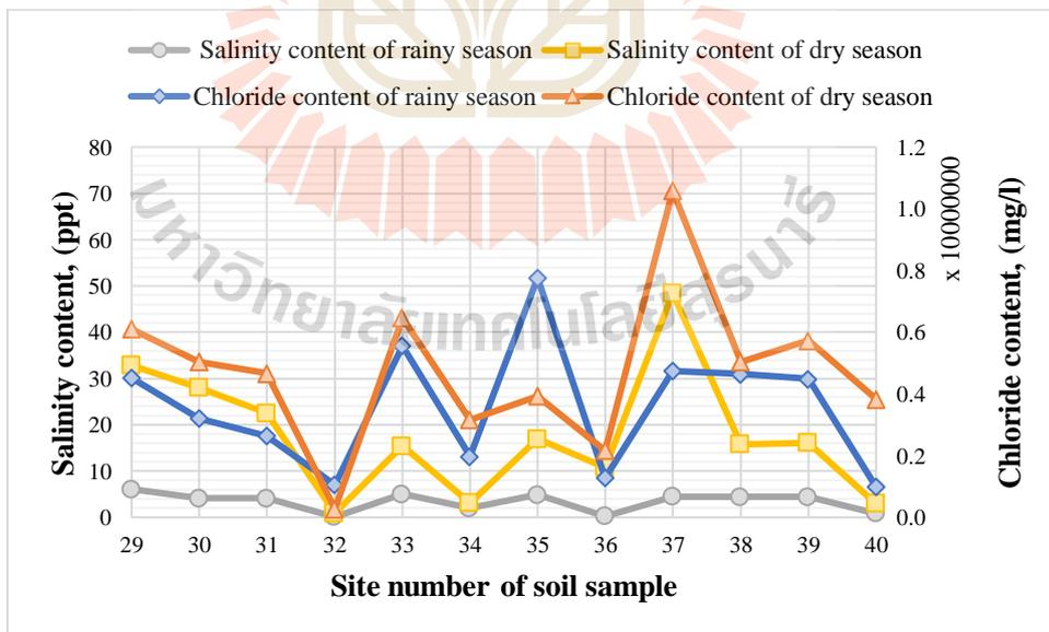
**Figure 4.20** The salinity content and chloride content of soil samples at Khong district.
