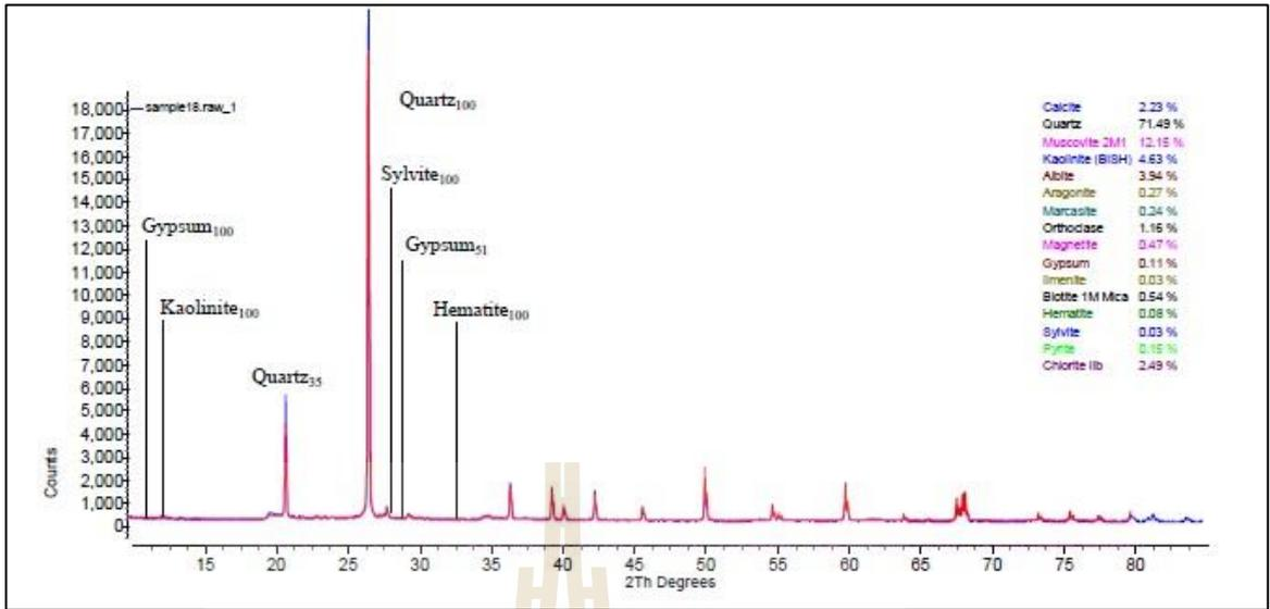
Figure B.15 Interpretation of X-Ray Diffractometer analysis from site number 18.
