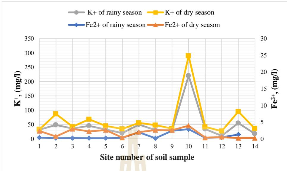
**Figure 4.29** Contents of potassium and iron ions of soil samples at Non Daeng district.
