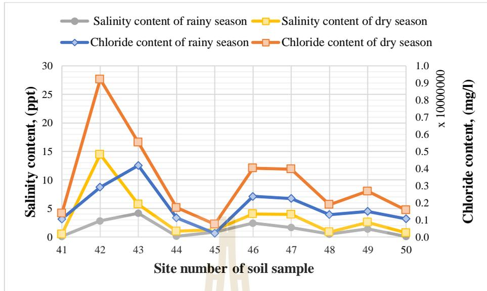
**Figure 4.21** The salinity content and chloride content of soil samples at Kham Sakae Saeng district.
