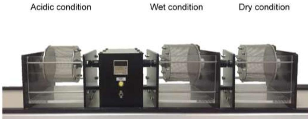
**Figure 4.1** Slake durability index test apparatus.
