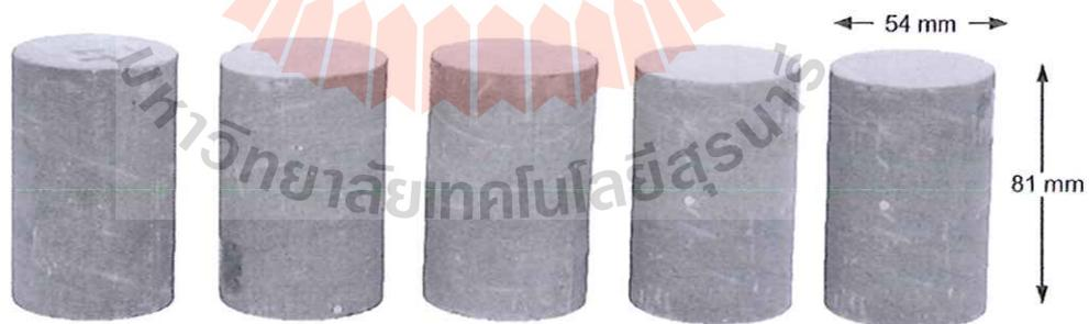
**Figure 3.6** Sao Khua sandstone specimens with core axis normal to bedding plane.
