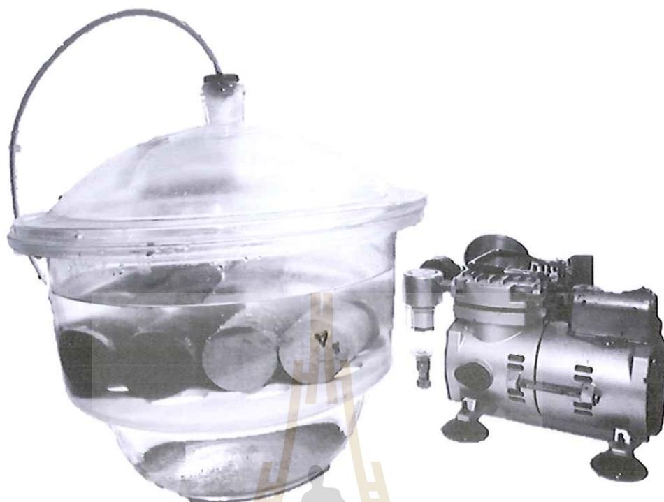
**Figure 3.7** Rock specimens saturated in vacuum-chamber at a negative pressure of 0.1 MPa for 48 hours.
