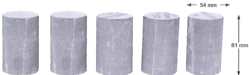
**Figure 3.4** Sao Khua sandstone specimens with core axis parallel bedding plane.
