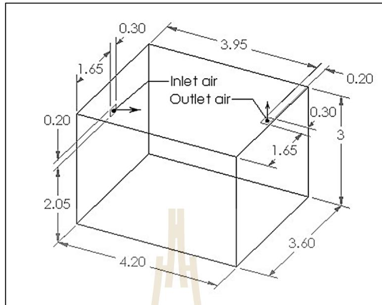
**Figure 3.1** Schematic drawing of the test room (m.).
