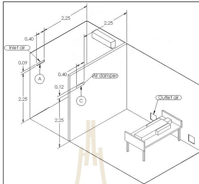
**Figure A.1** Case AC for  $3 \times 6 \times 3$  m room size.
