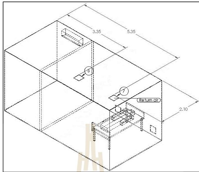
**Figure B.3** Case of air return channel 5-7 for  $3 \times 6 \times 3$  m room size.
