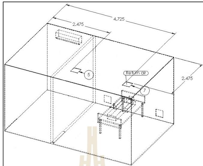
**Figure B.9** Case of air return channel 5-7 for  $3.5 \times 5.5 \times 3$  m room size.
