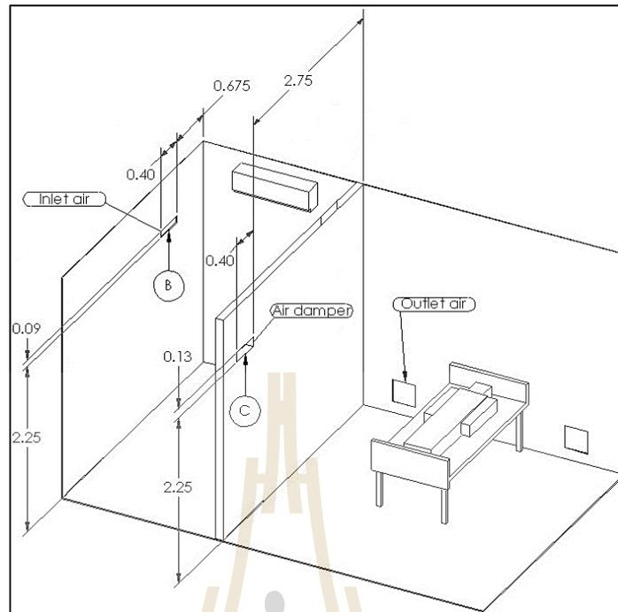
**Figure A.7** Case BC for  $3.5 \times 5.5 \times 3$  m room size.
