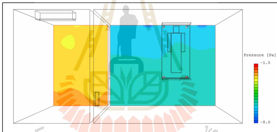
**Figure 4.15** Contour of pressure for case AC (6-9) of  $3 \times 6 \times 3$  m room size.
