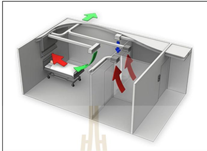
**Figure 1.1** Airborne Infection Isolation Room (AIIR).
