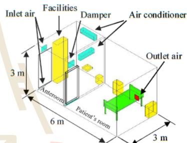
Figure 1 An airborne infection isolation room model
