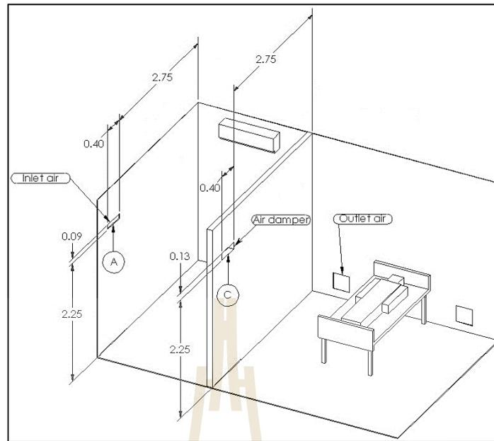
**Figure A.5** Case AC for  $3.5 \times 5.5 \times 3$  m room size.
