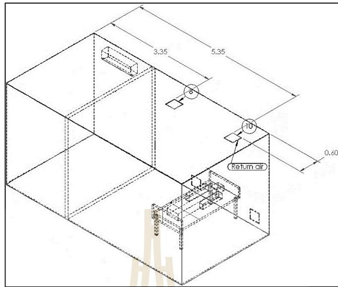
**Figure B.5** Case of air return channel 8-9 for  $3 \times 6 \times 3$  m room size.
