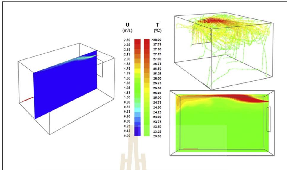
Figure 2.8 Path lines (temperature) in summer.
