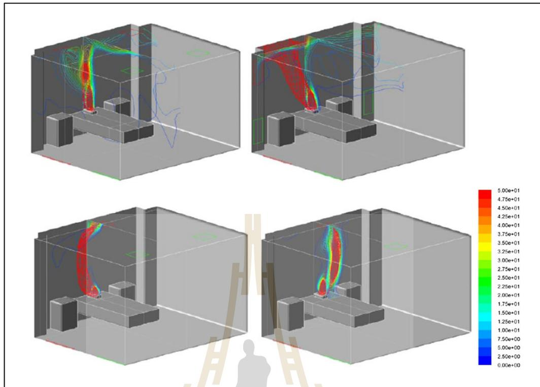
**Figure 2.15** Isosurface of 50 quanta  $m^3$  and quanta concentration in the planes  $x = 3$  m and  $y = 2$  m, for all the simulations with grille air supplies. Inlets are in green color and outlets are in red color (configuration 1 on the top left, configuration 12 on the top right, configuration 2 on the bottom left and configuration 5 on the bottom right).
