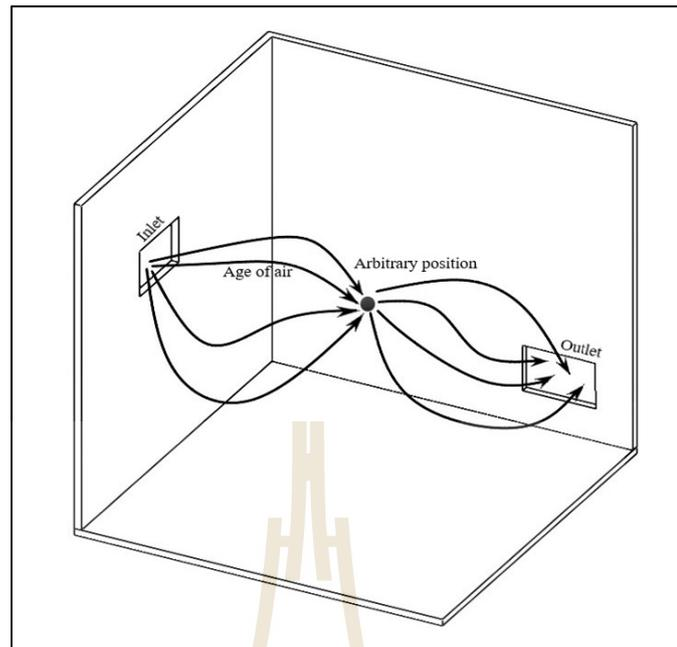
**Figure 2.3** Conceptual diagram of age of air.
