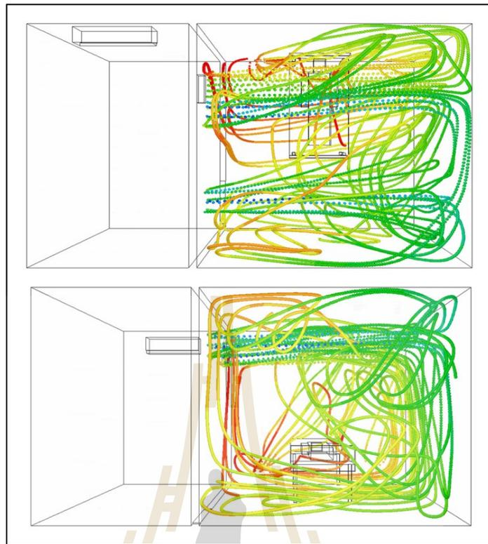
**Figure 4.10** The predicted SVE-3 distribution along the flow direction for case BD (1-2) (top) top view and (bottom) front view.
