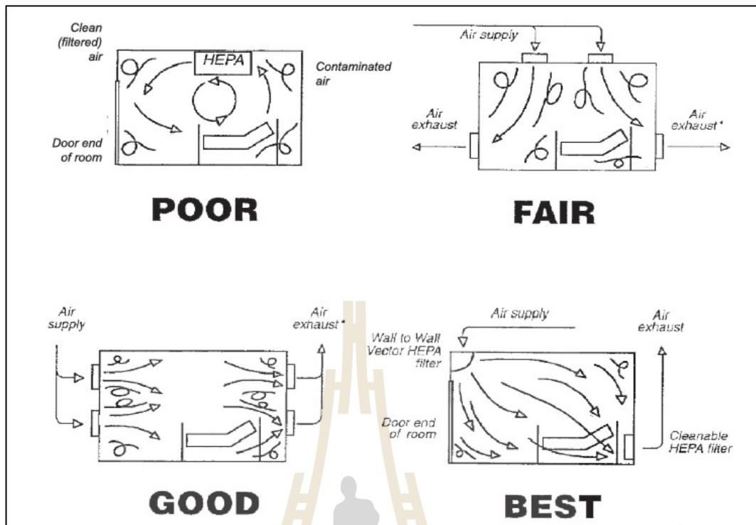
**Figure 2.2** Alignment of the inlet air and the suction air.
