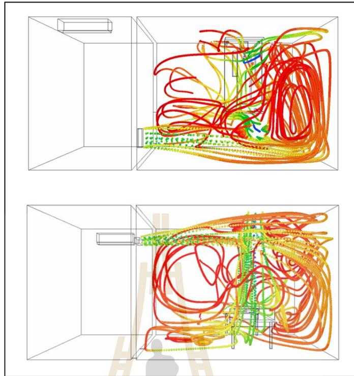
**Figure 4.2** The predicted SVE-3 distribution along the flow direction for case AC (6-9) (top) top view and (bottom) front view.
