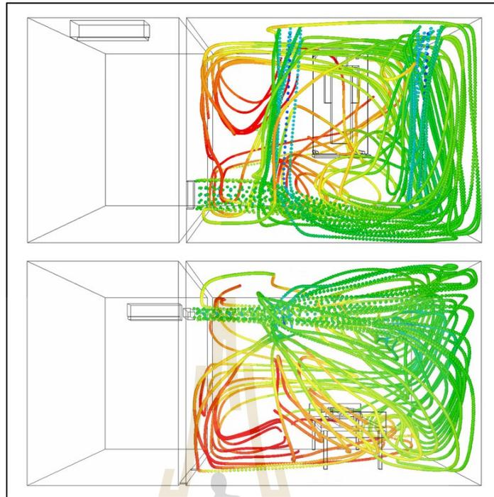
**Figure 4.4** The predicted SVE-3 distribution along the flow direction for case AC (11-12) (top) top view and (bottom) front view.
