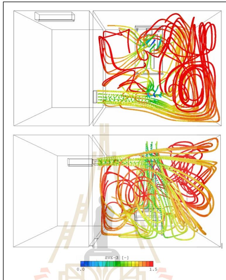
**Figure 4.7** The predicted SVE-3 distribution along the flow direction for case BC (11-12) (top) top view and (bottom) front view.
