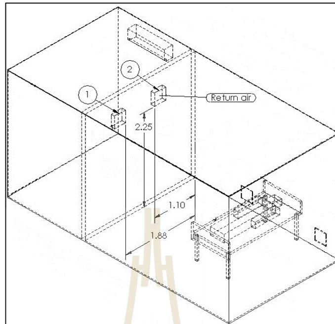
**Figure B.1** Case of air return channel 1-2 for  $3 \times 6 \times 3$  m room size.
