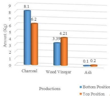
Fig. 8. Comparison of product amount obtain from each exhaust duct position.
