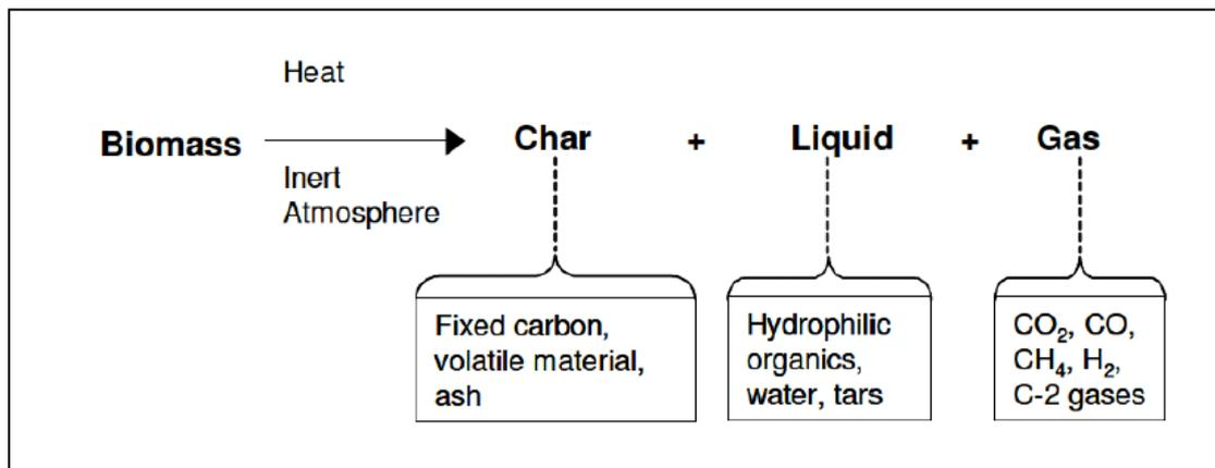
**Figure 2.12** A simple representation of pyrolysis process (Iberahim, 2013)
