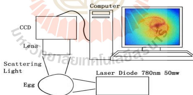
**Figure 2.2** Laser speckle imaging system (Yang et al., 2013)
