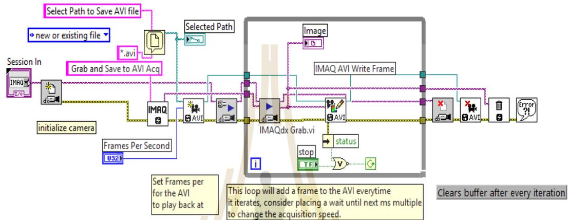
Figure A.1 Codes for recording video files
