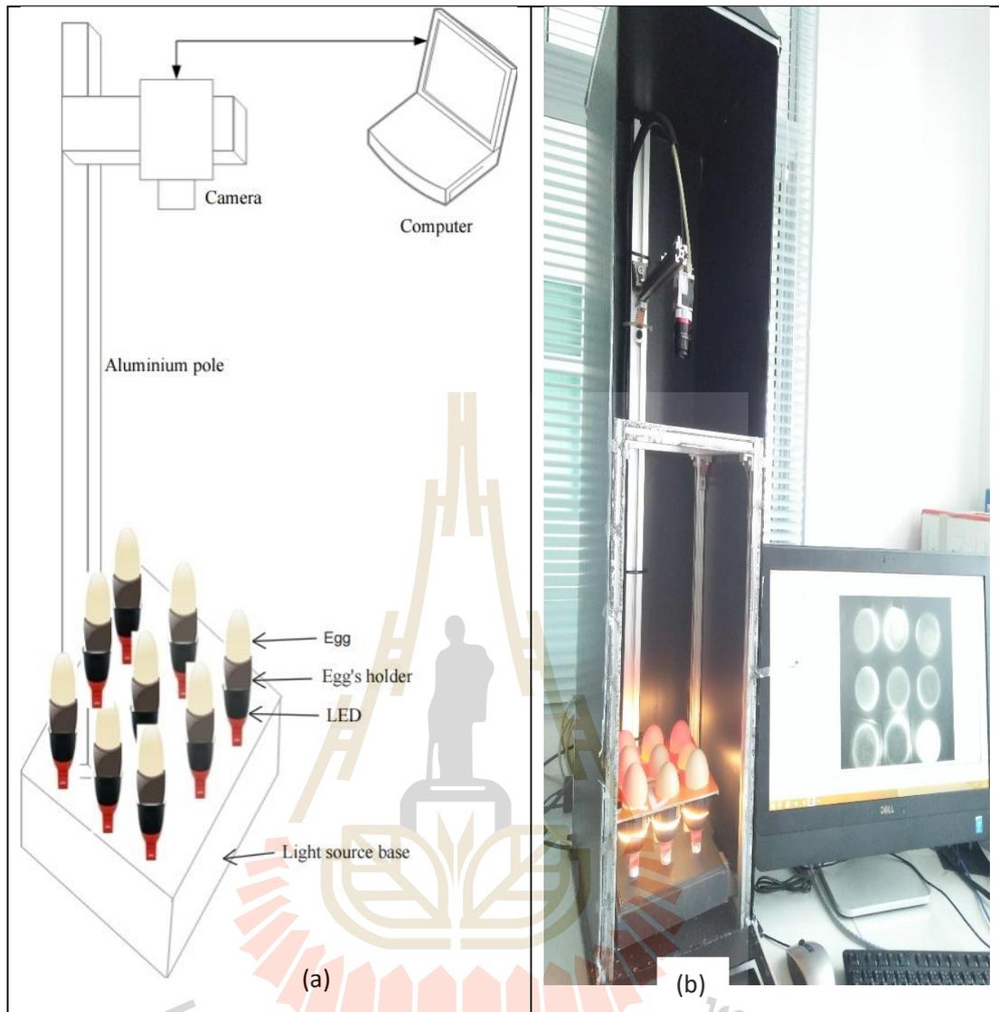
**Figure 3.1** Experimental setup (a) setup sketch (b) setup picture
