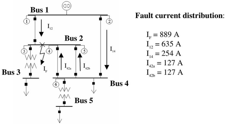
Fig. 2. Fault current distribution for the occurrence of fault at bus 2
