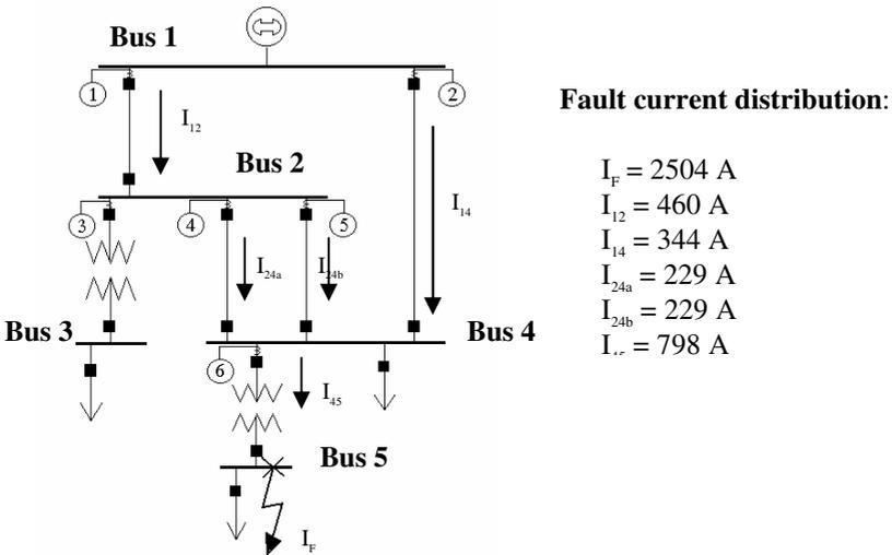
Fig. 3. Fault current distribution for the occurrence of fault at bus 5
