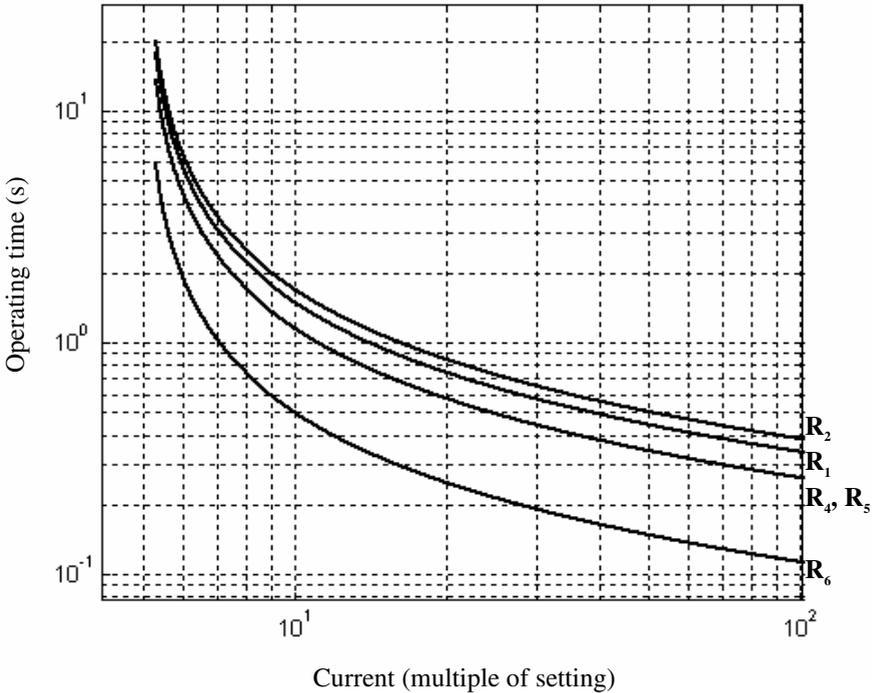
**Fig. 4.** Grading graph of the discriminated digital relay system
