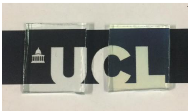
Figure 5.3 Photograph of bare glass (left) and 7 mol% FeCl 3 loaded ZnO film (right).
