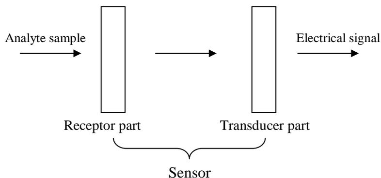
**Figure 1.1** Components of an optical chemical sensor.
