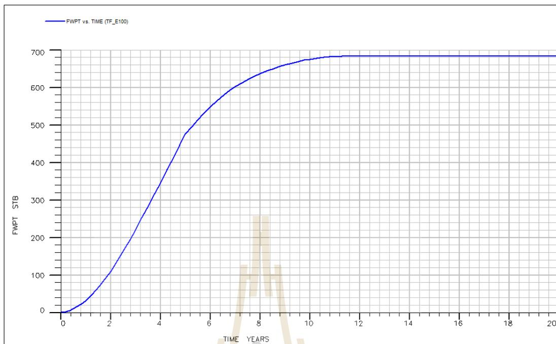
**Figures D.146** Water production total Vs. time of model case 18
