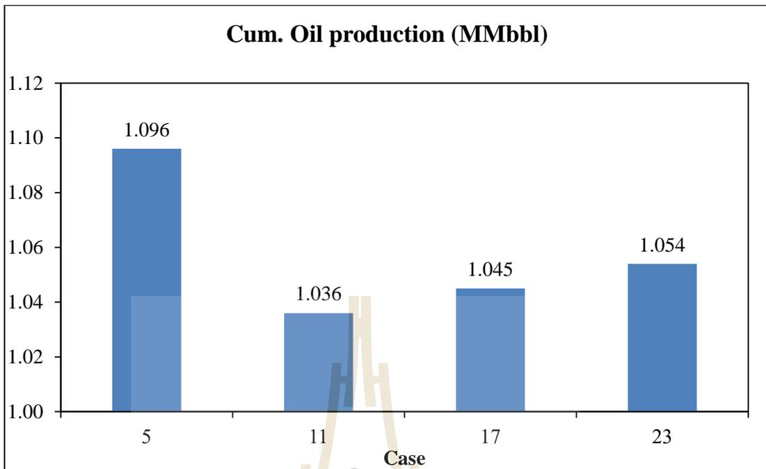
**Figure 4.17** Cumulative oil production is use inject rate 150 bbl/d in fifth year to inject
