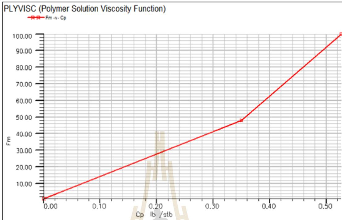
**Figure 3.7** Polymr solution viscosity function graph display
