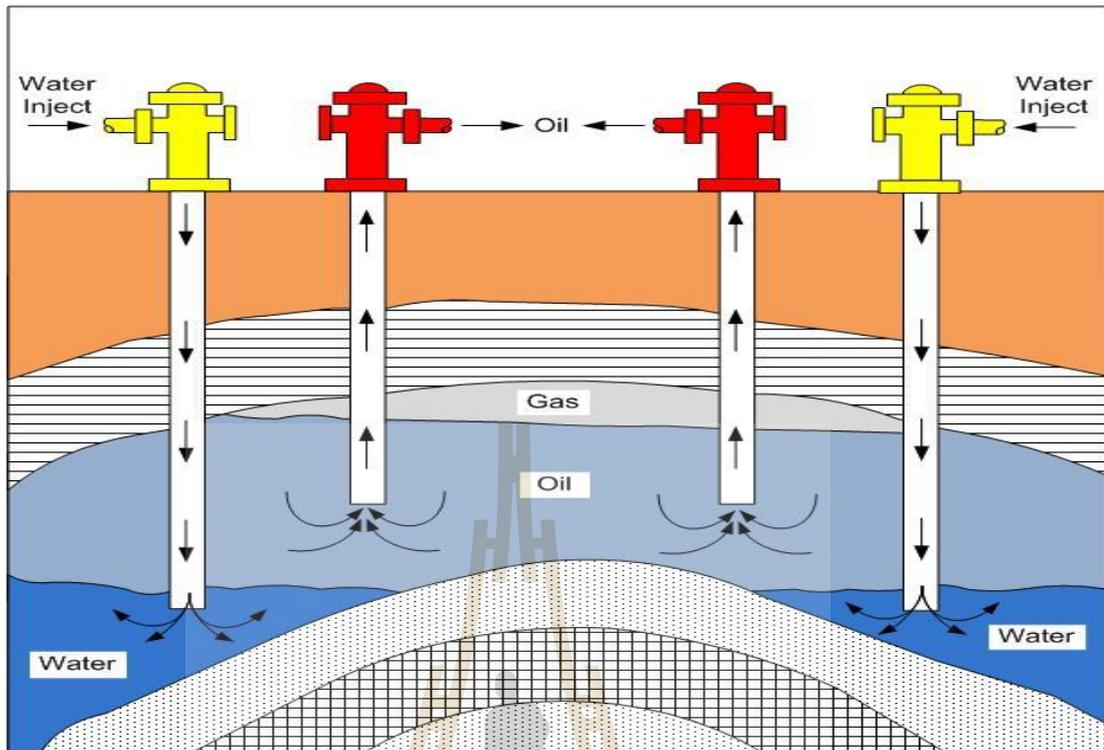
**Figure 2.5** Water flooding method showing two water injection wells and two well productions (Thongsumrit, 2012)
