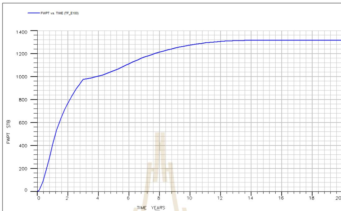
**Figures D.182** Water production total Vs. time of model case 22
