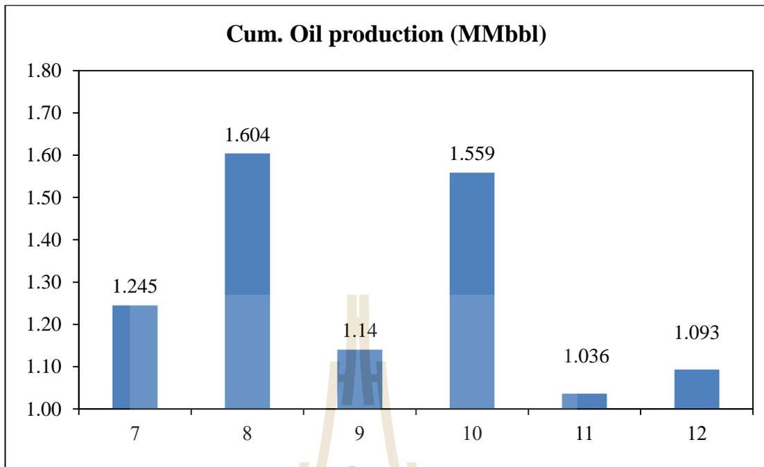
**Figure 4.3** Cumulative oil production in polymer flooding at concentration 600 ppm
