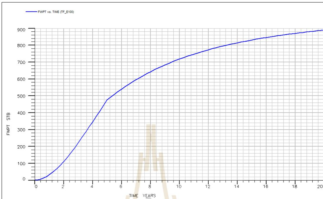
**Figures D.137** Water production total Vs. time of model case 17
