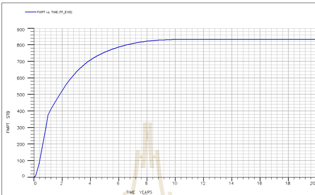
**Figures D.110** Water production total Vs. time of model case 14
