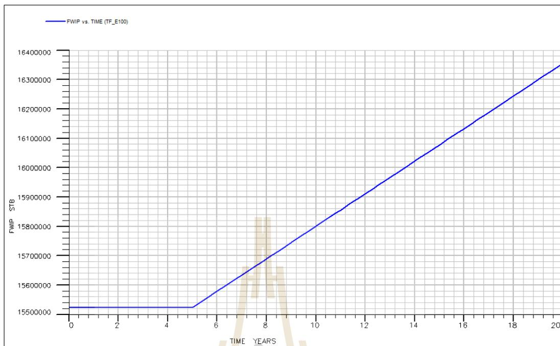
**Figures D.189** Water in place Vs. time of model case 23
