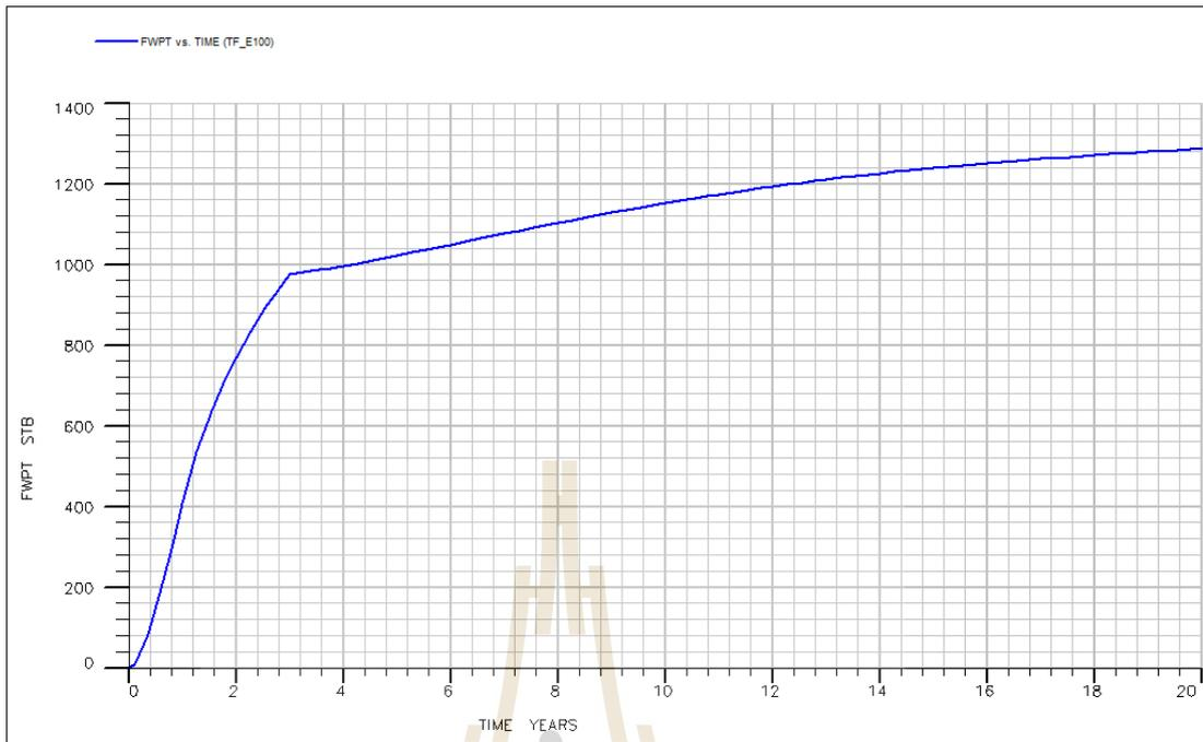
**Figures D.65** Water production total Vs. time of model case 9
