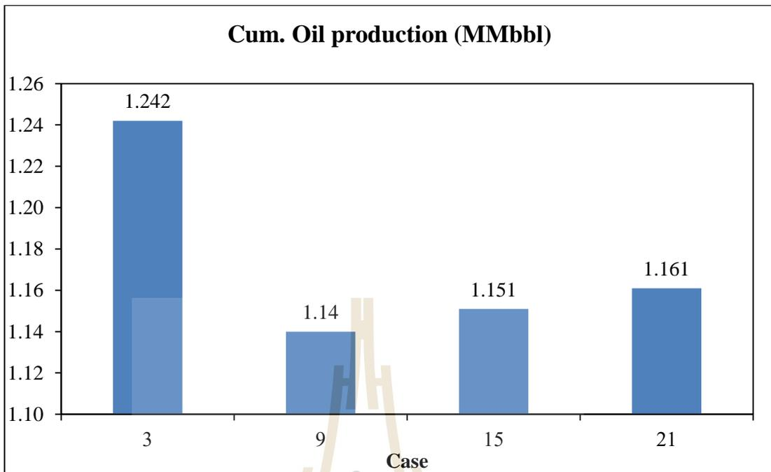
**Figure 4.13** Cumulative oil production is use inject rate 150 bbl/d in third year to inject
