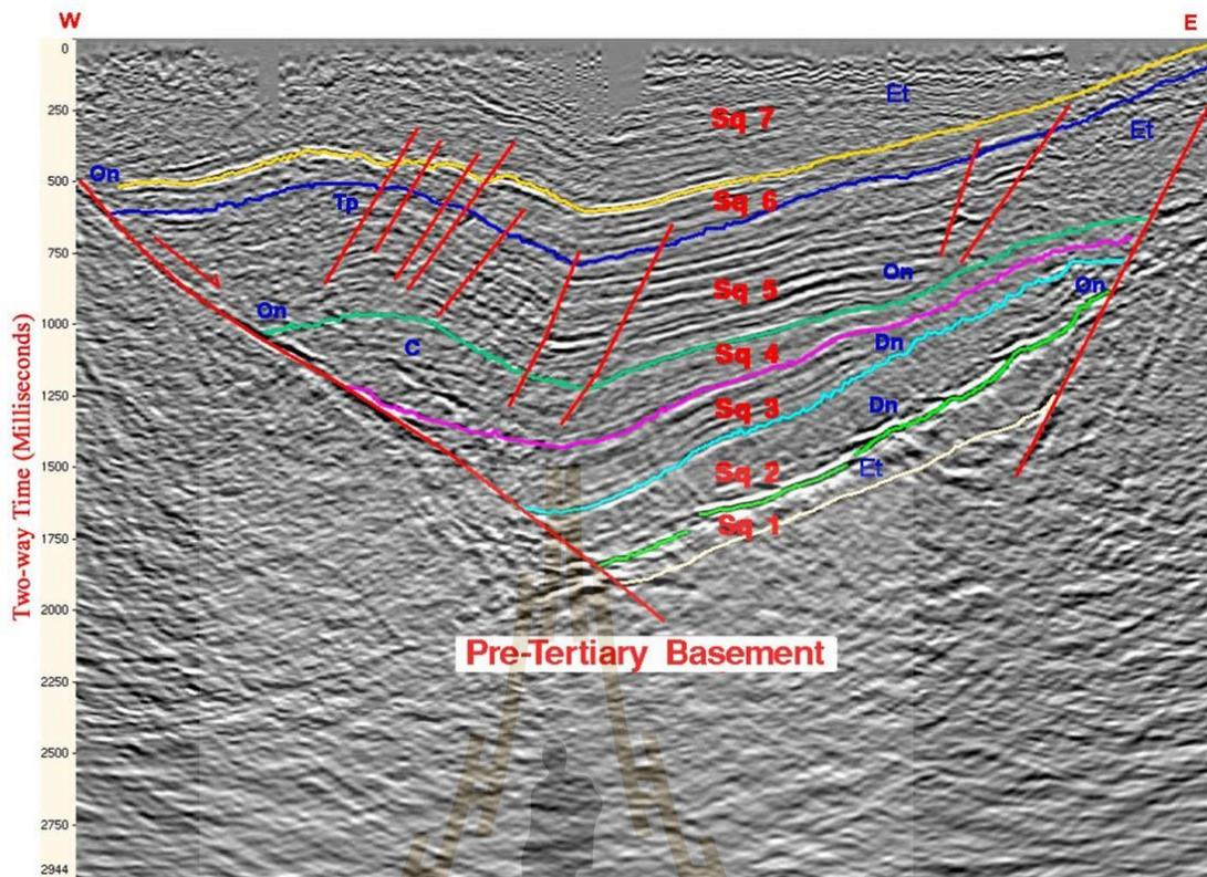
**Figure 2.4** Interpretation of a seismic profile across the study area with 8 seismic units Basement and Sq1 to Sq7. On = onlap; Dn = downlap; Tp = Toplap; Et = erosional truncation; C = Clinoform
