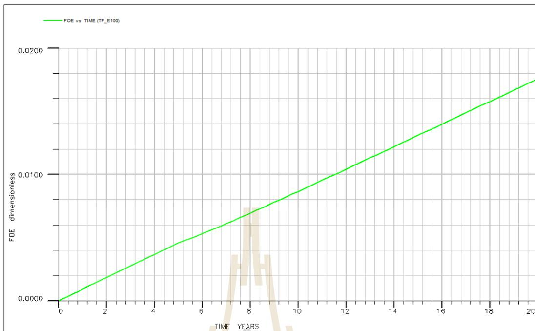
**Figures D.195** Oil efficiency Vs. time of model case 23
