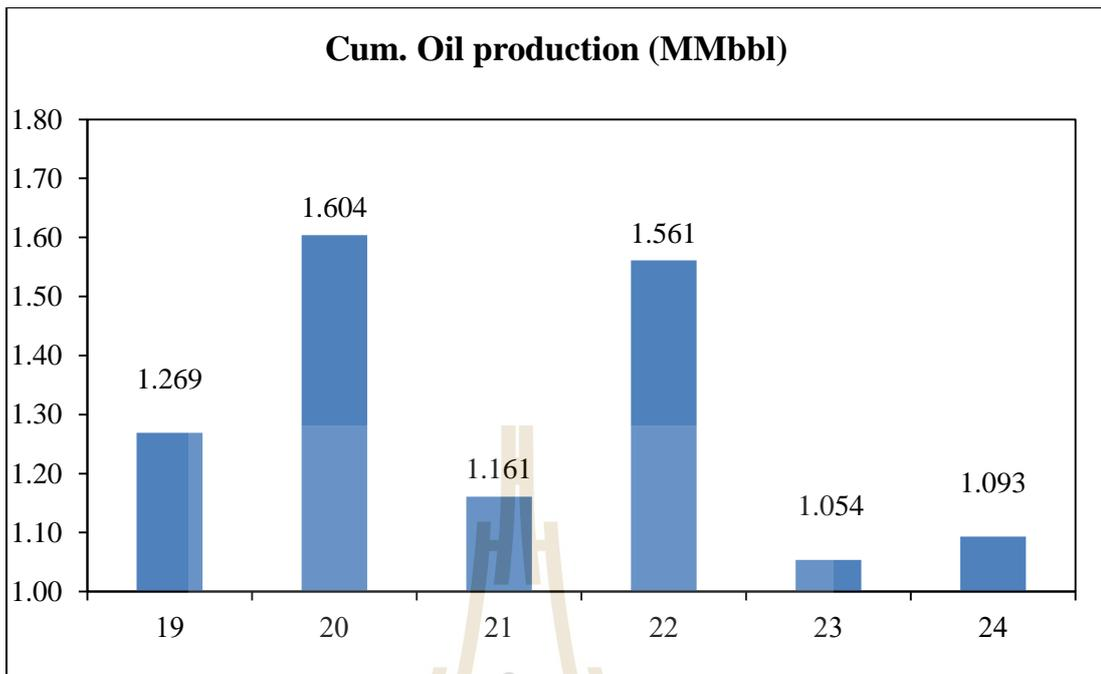
**Figure 4.7** Cumulative oil production in polymer flooding at concentration 1,500 ppm
