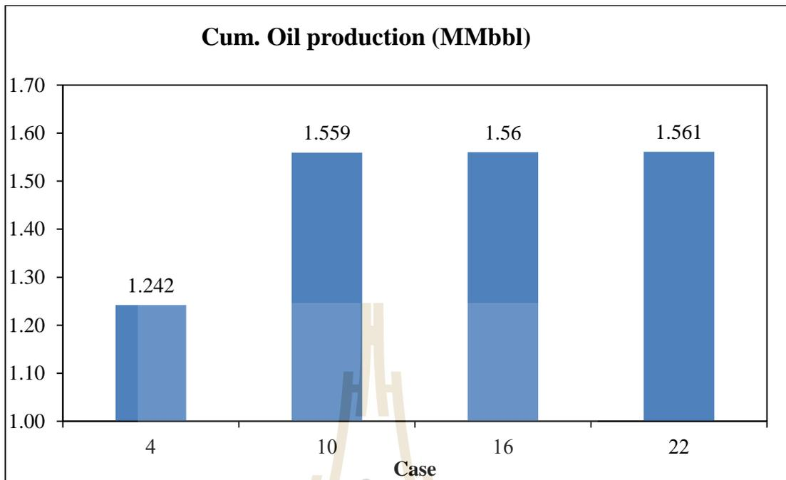
**Figure 4.15** Cumulative oil production is use inject rate 300 bbl/d in third year to inject
