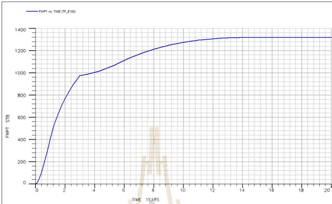
**Figures D.128** Water production total Vs. time of model case 16
