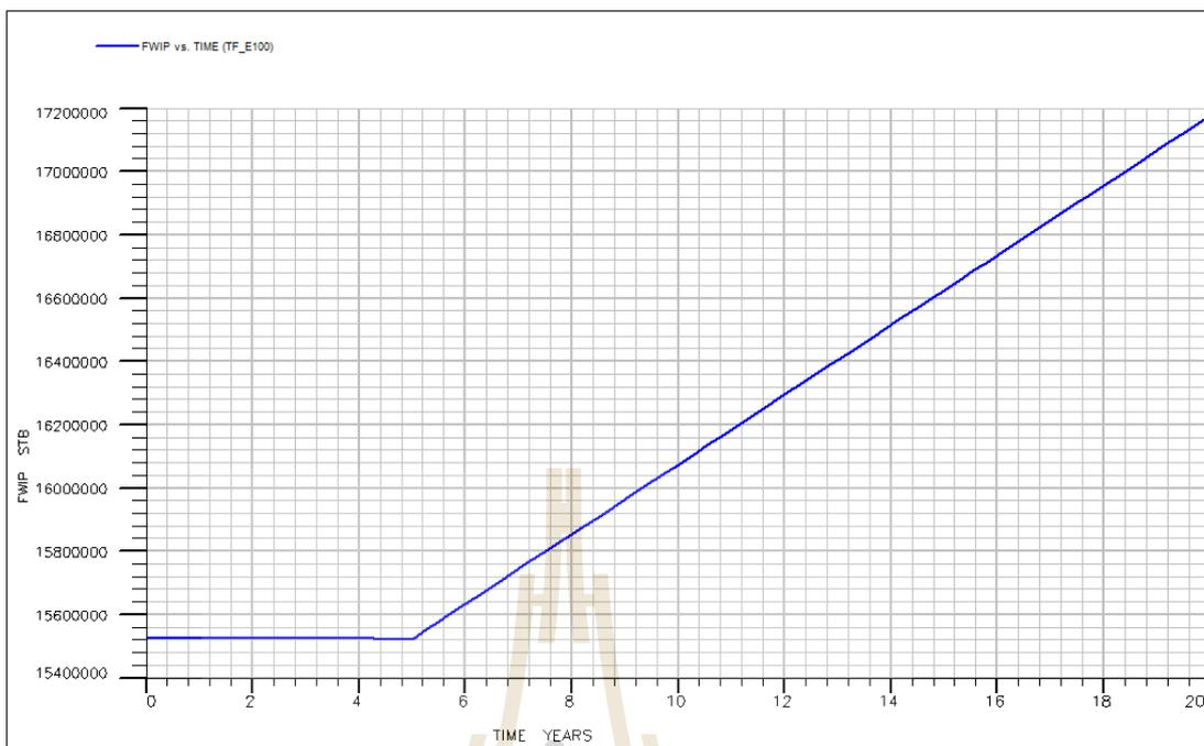
**Figures D.198** Water in place Vs. time of model case 24
