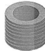
Figure 2: Layer contours of sliced cylinder model
