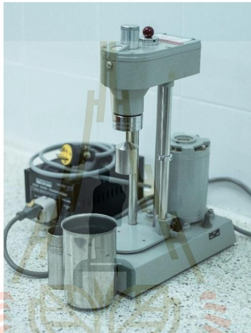
**Figure 3.6** Fann model 35SA viscometer.
