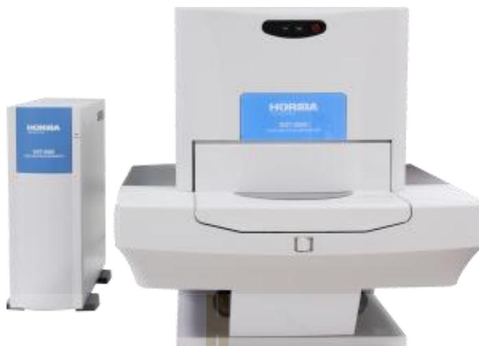
**Figure 3.4** Horiba (XGT-5200) X-ray fluorescence.
