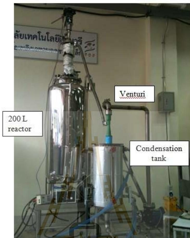
**Figure 4.7** Experimental setup for extractive fermentation of ethanol from molasses using vacuum fractionation technique. A venturi was used to generate vacuum condition and the vapor distillate ethanol was condensed.
