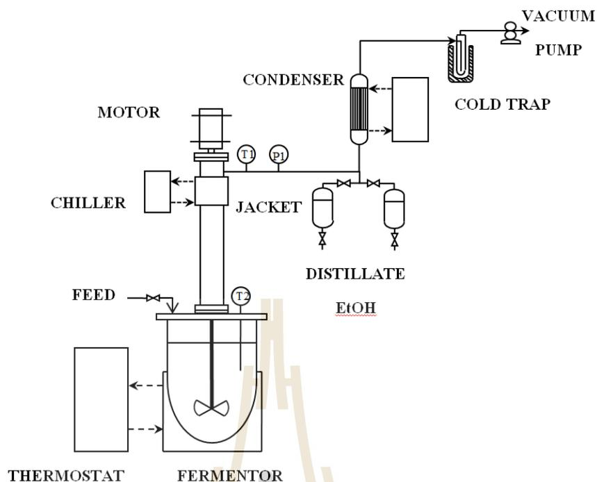
**Figure 3.1** Schematic diagram and experimental set up of extractive fermentation of ethanol using vacuum fractionation technique.
