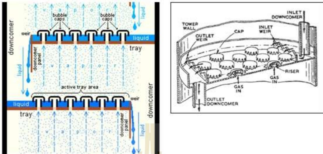
Figure 2.4 Internal structure of cap tray fractionating column (ACS, 2006).
