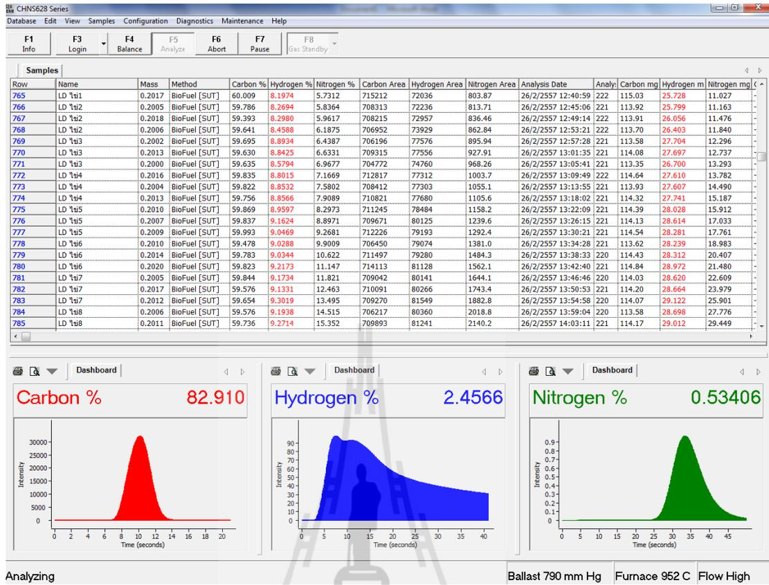
**Figure C2** The main window displays of the LECO CHN628 Series Elemental Analyzer and CHN628 series parameters.
