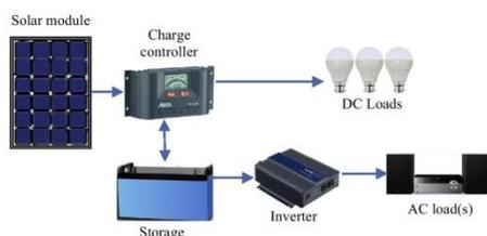
Fig. 2. A stand-alone solar PV system with dc and ac loads.
