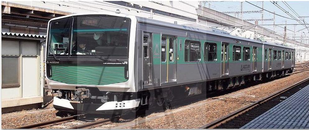
**Figure 2.8** JR East Catenary and battery hybrid railcar EV-E301(Shiraki, et al., 2015).
