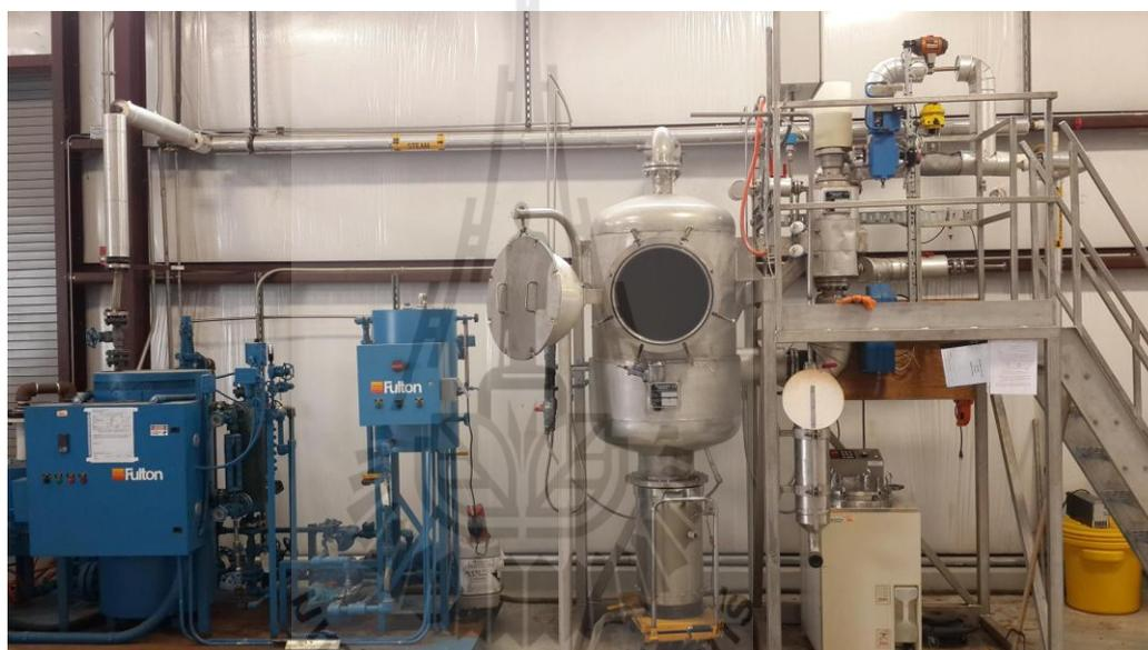
**Figure 5.4** Showing the steam gun that used for production of hemicellulose hydrolysate.
