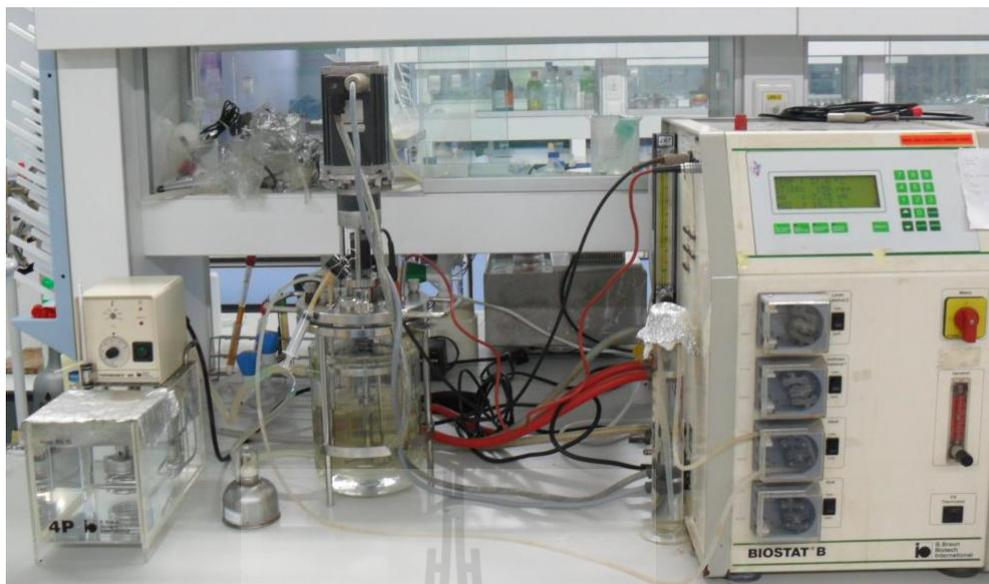
**Figure 3.2** A 2-L bioreactor apparatus.
