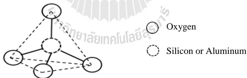
**Figure 2.1** Representation of  $[\text{SiO}_4]^{4-}$  or  $[\text{AlO}_4]^{5-}$  tetrahedral (Dyer, 1988).
