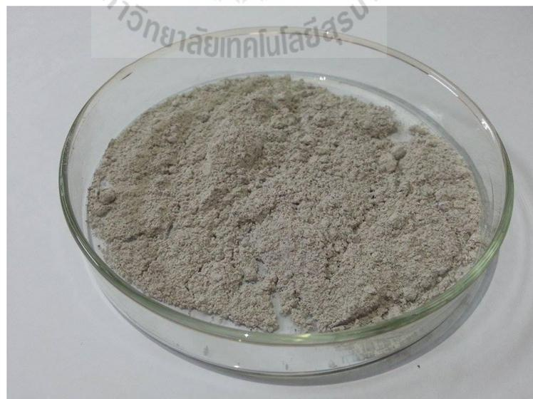
**Figure 3.6** Rock powder prepared for XRD analysis
