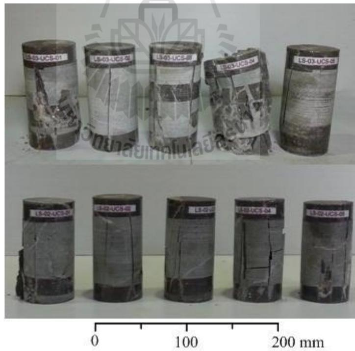
**Figure 4.4** Example of the rock samples with failed under loading from uniaxial compressive strength testing
