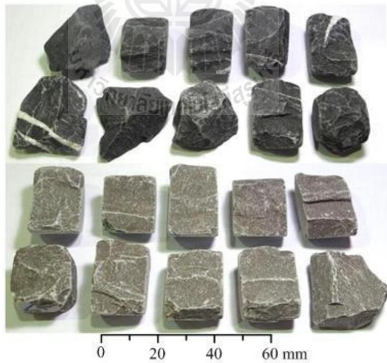
**Figure 4.8** Examples of the post-tested specimens from slake durability index test
