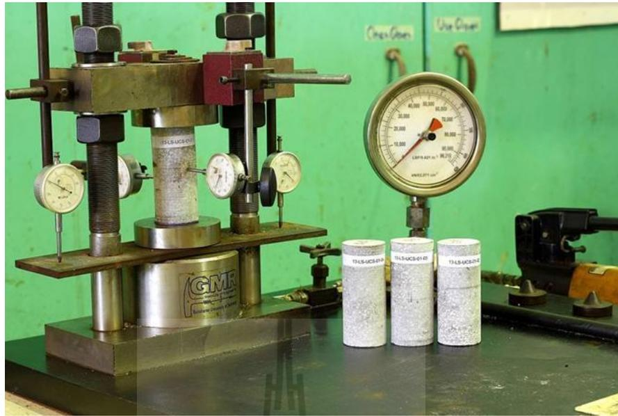
**Figure 4.3** Uniaxial compressive strength test device
