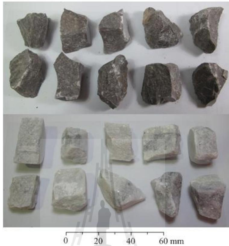
**Figure 3.4** Examples of irregular shape specimens prepared for slake durability index test and Los Angeles abrasion and impactation test
