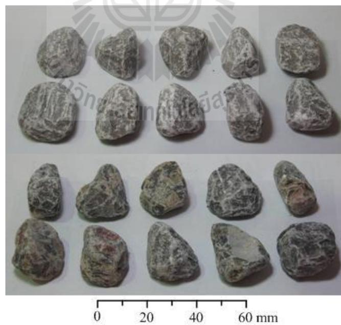
**Figure 4.10** Examples of the specimens after testing of Los Angeles abrasion and impact test
