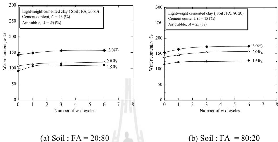
**Figure 4.6** Relationship between  $w$  and  $N$  for (a) Soil : FA = 20:80 and (b) Soil : FA = 80:20.
