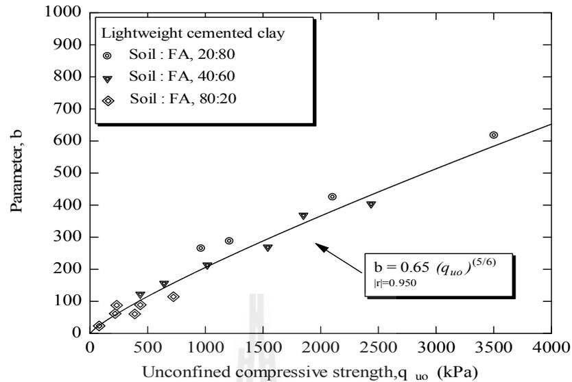
**Figure 4.10** Relationship between  $b$  and  $q_{u0}$  for soil : FA tested.
