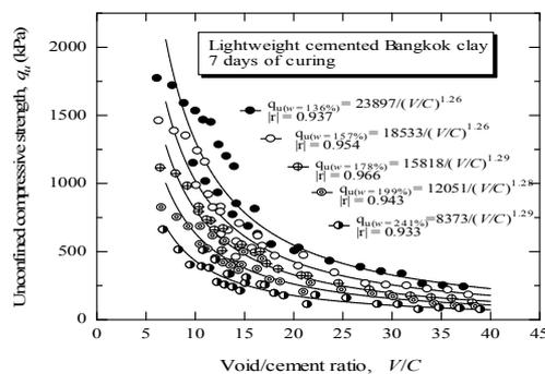
**Figure 2.3** Analysis of strength development in lightweight cemented Bangkok clay using  $V/C$  (Horpibulsuk et al., 2012b).
