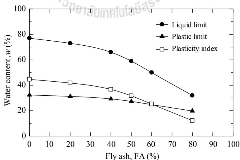
**Figure 3.2** Index properties of clay-FA mixture.
