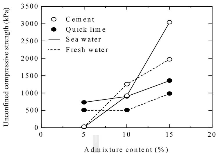
**Figure 2.2(b)** Relationship between unconfined compressive strength and admixture content (after Miura et al., 1988).
