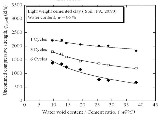
**Figure 4.5** Relationship between  $q_u(w-d)$  and  $wV/C$ .
