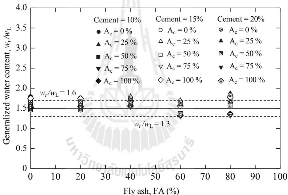
**Figure 3.9** Determination of  $w_t$  in terms of  $w_L$ .
