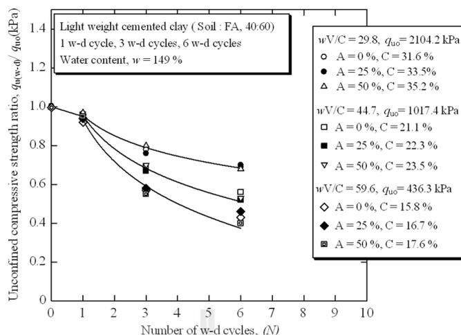
**Figure 4.8** Normalized strength,  $q_{u(w-d)}/q_{u0}$  versus  $N$  relationship
