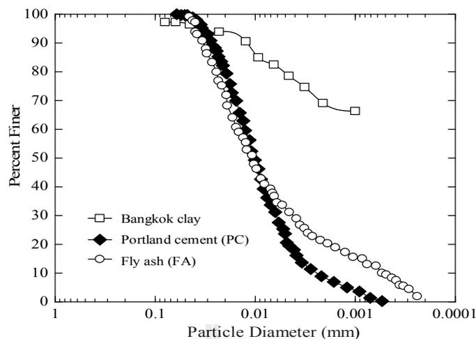
**Figure 3.1** Grain size distribution of Bangkok clay, PC and FA.
