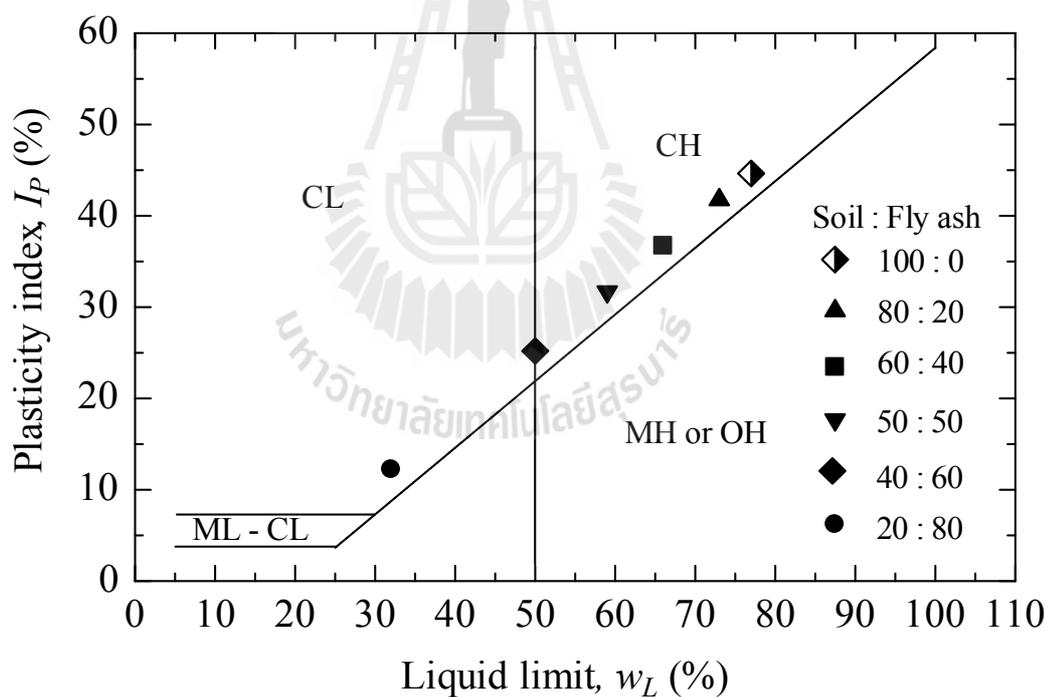
**Figure 3.3** State of water content of clay-FA mixture compared with A-line
