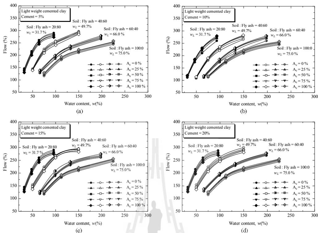
**Figure 3.7** Relationship between flowability and water content for different replacement ratios.
