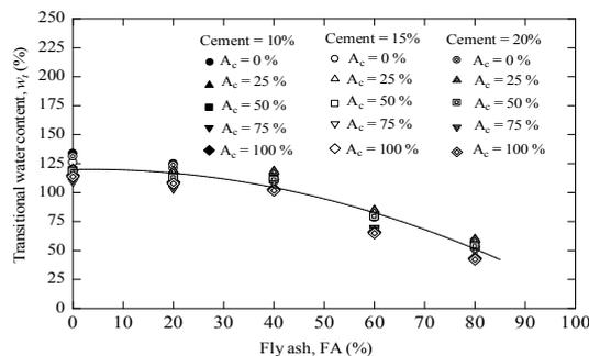
**Figure 3.5** Relationship between transitional water content and FA replacement for different air contents and cement contents.
