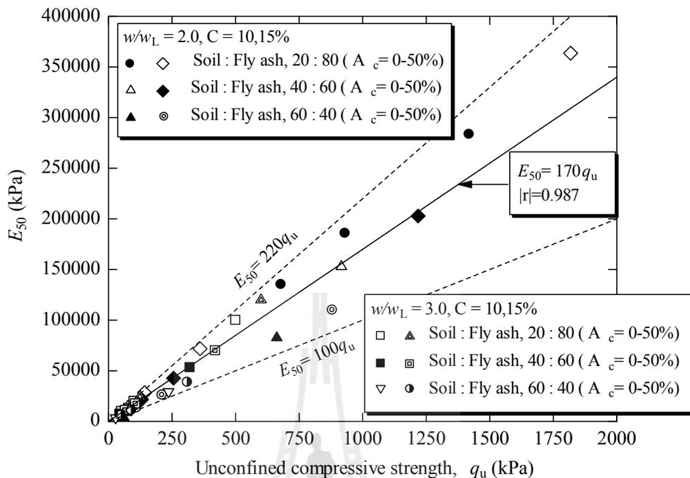
**Figure 3.14** Relationship between  $E_{50}$  and  $q_u$  of lightweight cellular cemented clay.
