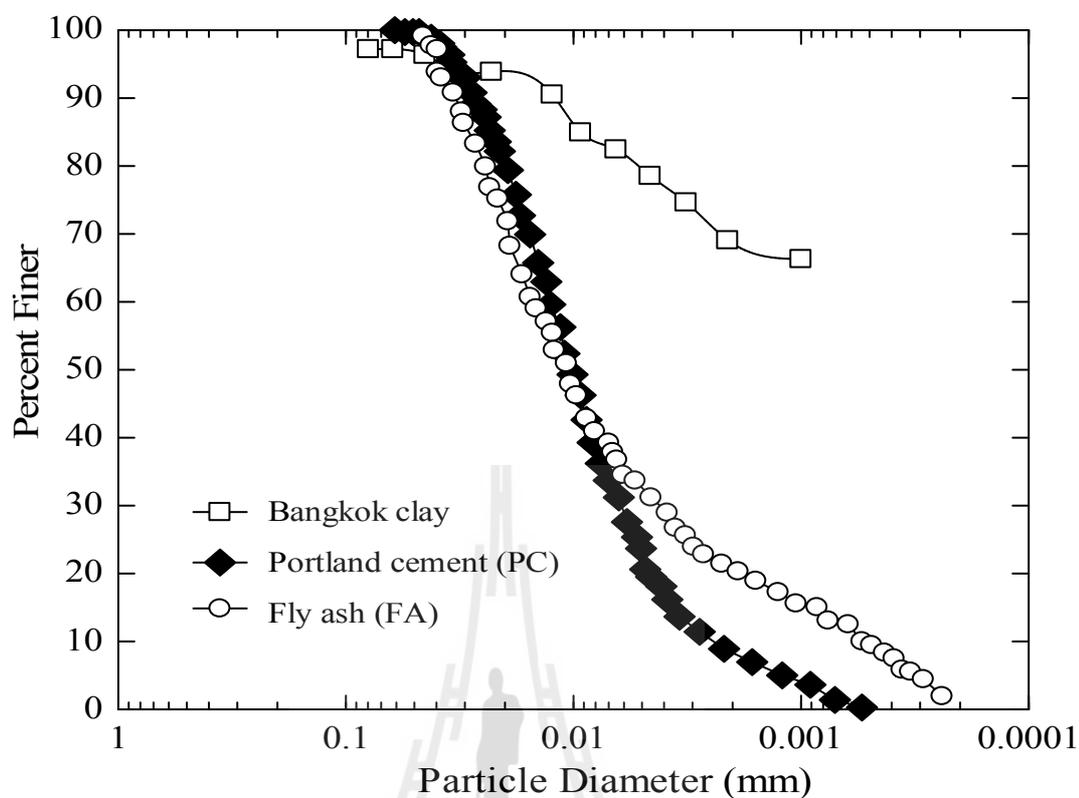
**Figure 4.1** Grain size distribution of clay, PC, and FA.
