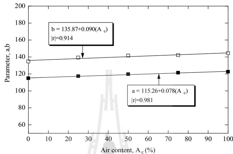
**Figure 3.11** Determination of  $a$  and  $b$  values in terms of  $A_c$ .
