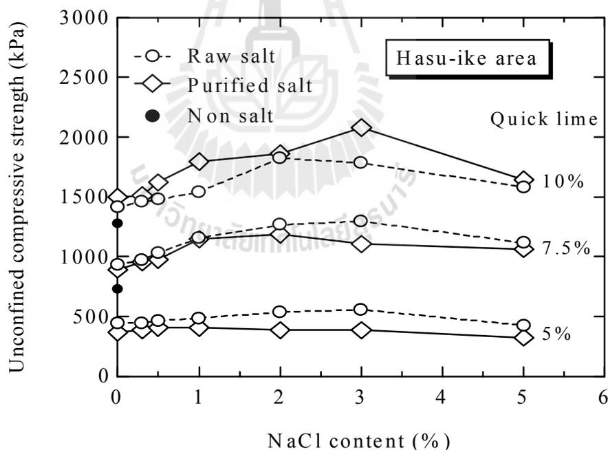
**Figure 2.2(a)** Influence of NaCl content on the quick lime improvement of Ariake clay (after Miura et al., 1988).
