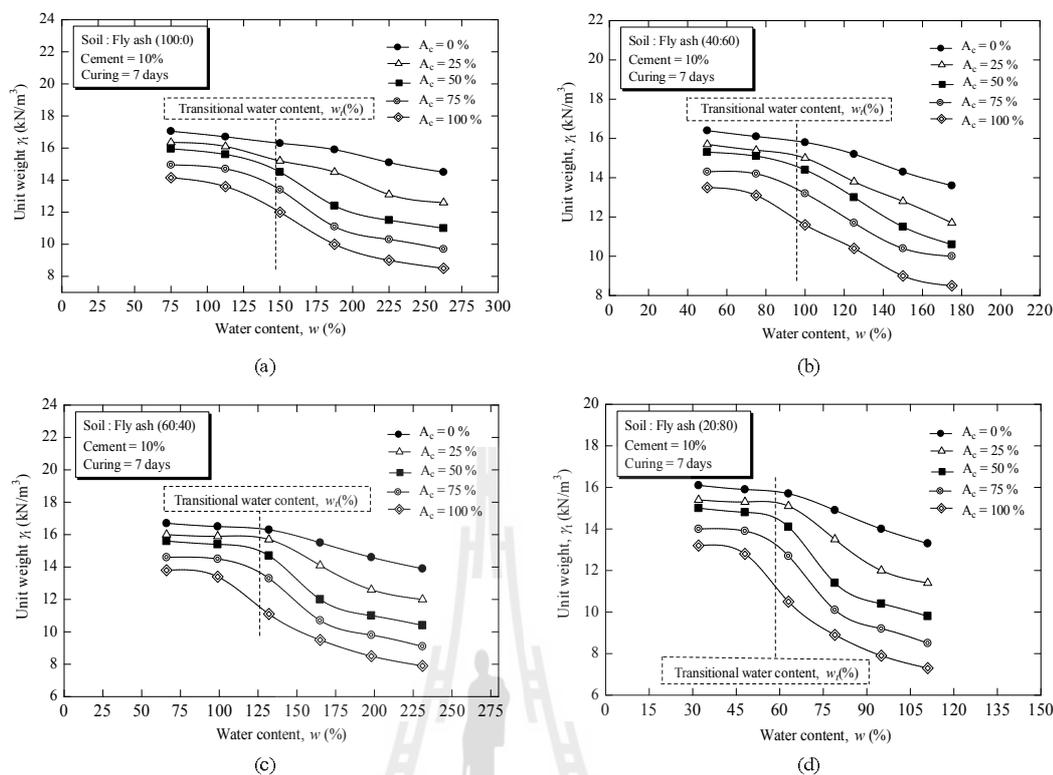
**Figure 3.4** Relationship between unit weight and water content at different air contents.
