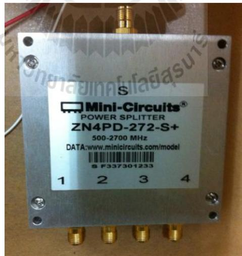
**Figure 5.13** Photograph of power splitter/combiner.
