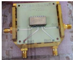
**Figure 5.3** Photograph of phase shifter.
