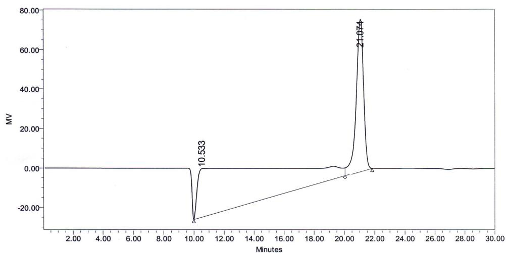
**Figure 14C.** HPLC Chromatogram of 2 mg/ml standard D-lactic acid Vertisep™ OA HPLC with a 0.005M H<sub>2</sub>SO<sub>4</sub> mobile phase and a refractive index detector.
