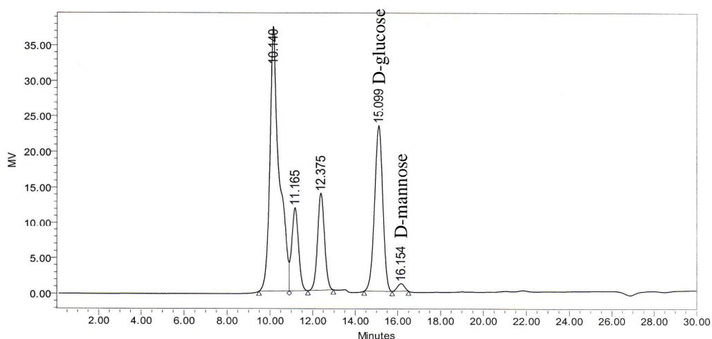
**Figure 2C.** HPLC Chromatogram of partial hydrolyzed exopolysaccharide from *Lactobacillus* sp. FKU23 cultivated in MRS broth containing 4.5% of white sugar from sugar cane with initial pH of 7.0 at 30°C. Sample injection volume was 100  $\mu$ l. Chromatographic run time was 30 min.
