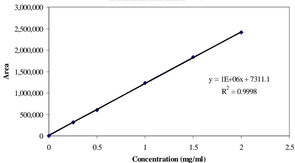
**Figure 6B.** Standard curve of standard D-lactic acid using Vertisep™ OA HPLC with a 0.005 M H<sub>2</sub>SO<sub>4</sub> mobile phase and a refractive index detector.
