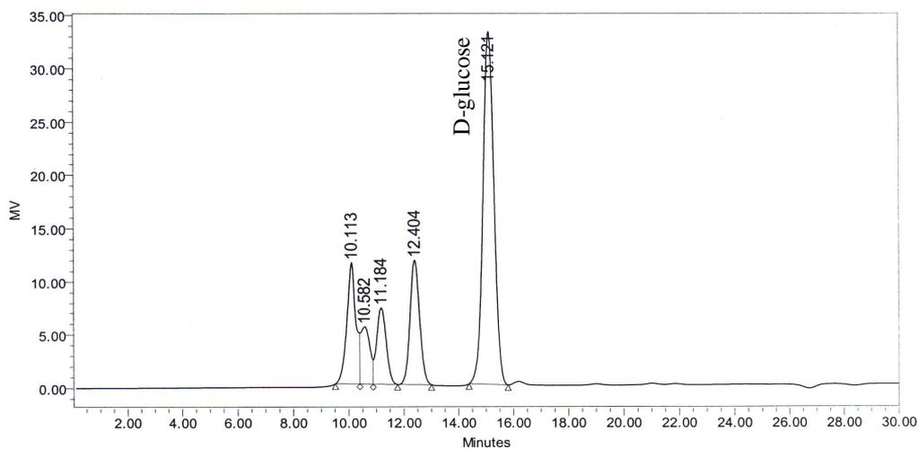
**Figure 8C.** HPLC Chromatogram of partial hydrolyzed exopolysaccharide from *Weissella* sp. PSMS4-4 cultivated in MRS broth containing 5% of white sugar from sugar cane with initial pH of 7.0 at 30°C. Sample injection volume was 100  $\mu$ l. Chromatographic run time was 30 min.
