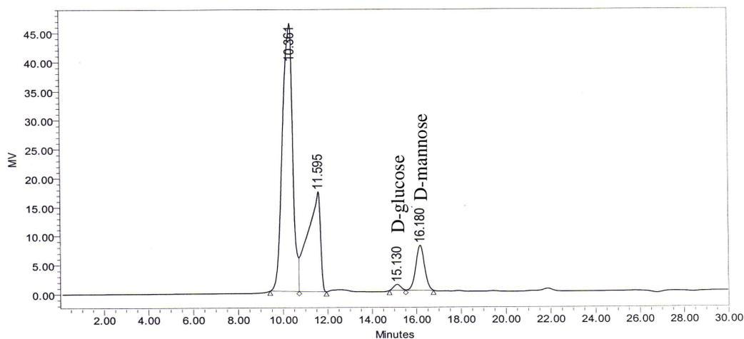
**Figure 4C.** HPLC Chromatogram of partial hydrolyzed exopolysaccharide from *Streptococcus* sp. I5 cultivated in MRS broth containing 3.5% of white sugar from sugar cane with initial pH of 6.0 at 40°C. Sample injection volume was 100  $\mu$ l. Chromatographic run time was 30 min.
