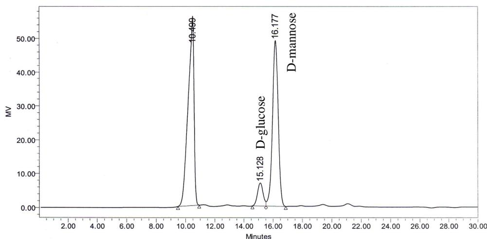
**Figure 9C.** HPLC Chromatogram of partial hydrolyzed exopolysaccharide from *Weissella* sp. PSMS4-4 cultivated in MRS broth containing 2% of glucose with initial pH of 6.2 at 30°C. Sample injection volume was 100  $\mu$ l. Chromatographic run time was 30 min.
