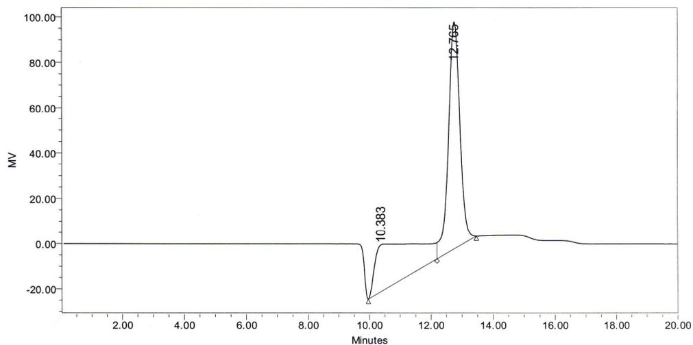
**Figure 15C.** HPLC Chromatogram of 2 mg/ml standard D-sucrose (analytical grade) using Vertisep™ OA HPLC with a 100% water mobile phase and a refractive index detector.
