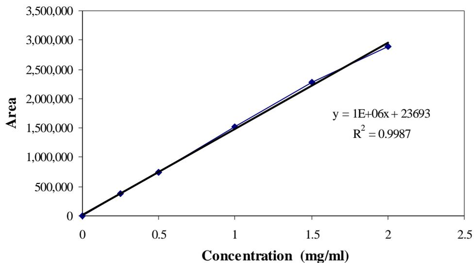
**Figure 3B.** Standard curve of standard D-glucose using Vertiseq™ OA HPLC with a 100% water mobile phase and a refractive index detector.
