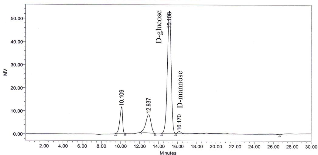
**Figure 7C.** HPLC Chromatogram of partial hydrolyzed exopolysaccharide from *Leuconostoc* sp. PSMS1-5 cultivated in MRS broth containing 4.5% of white sugar from sugar cane with initial pH of 5.0 at 37°C. Sample injection volume was 100  $\mu$ l. Chromatographic run time was 30 min.
