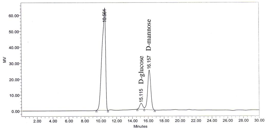
**Figure 1C.** HPLC Chromatogram of partial hydrolyzed exopolysaccharide from *Lactobacillus salivarius* C56 cultivated in MRS broth containing 2% of glucose with initial pH of 6.2 at 37°C for 48 h. Sample injection volume was 100  $\mu$ l. Chromatographic run time was 30 min.
