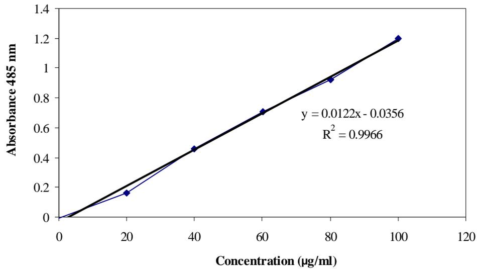
**Figure 1B.** Standard curve of glucose according to phenol-sulfuric acid method (Dubois *et al.*, 1956).
