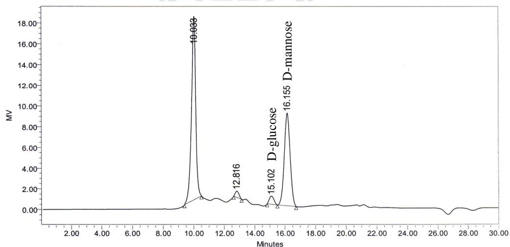
**Figure 5C.** HPLC Chromatogram of partial hydrolyzed exopolysaccharide from *Streptococcus* sp. I5 cultivated in MRS broth containing 2% of glucose with initial pH of 6.2 at 37°C. Sample injection volume was 100  $\mu$ l. Chromatographic run time was 30 min.
