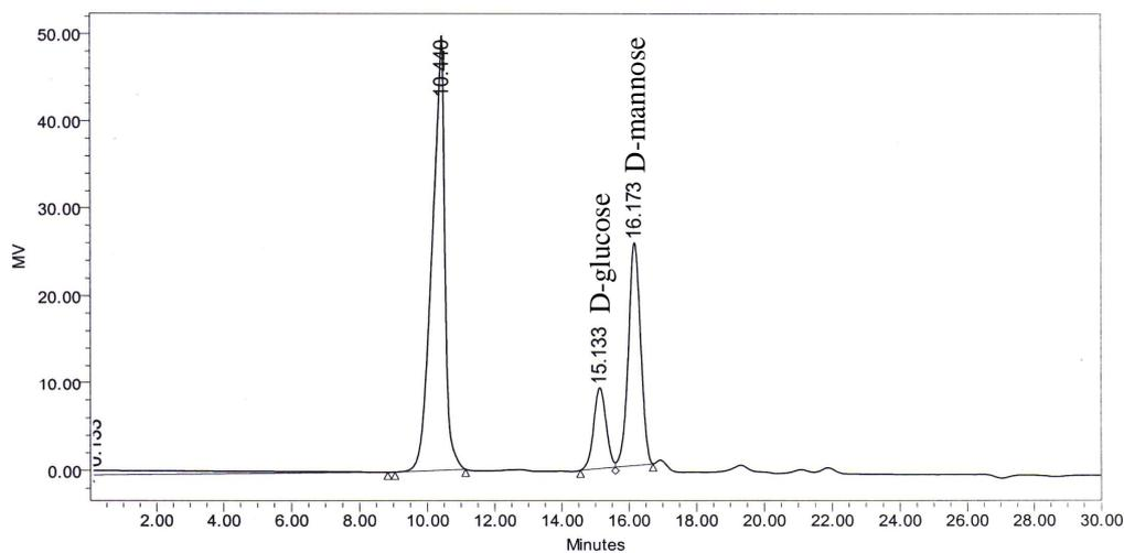
**Figure 10C.** HPLC Chromatogram of partial hydrolyzed exopolysaccharide from *Lactobacillus* sp. RMS3-1 cultivated in MRS broth containing 3% of white sugar from sugar cane with initial pH of 8.0 at 35°C. Sample injection volume was 100  $\mu$ l. Chromatographic run time was 30 min.
