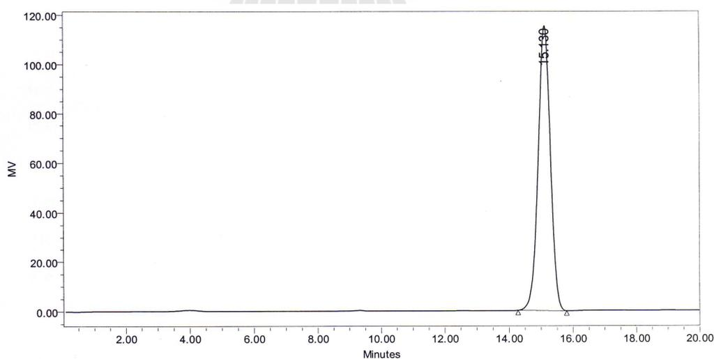
**Figure 11C.** HPLC Chromatogram of 2 mg/ml standard D-glucose using Vertisep™ OA HPLC with a 100% water mobile phase and a refractive index detector.
