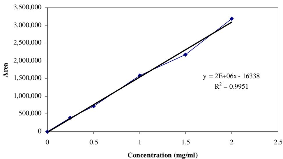
**Figure 4B.** Standard curve of standard D-mannose using Vertiseq™ OA HPLC with a 100% water mobile phase and a refractive index detector.
