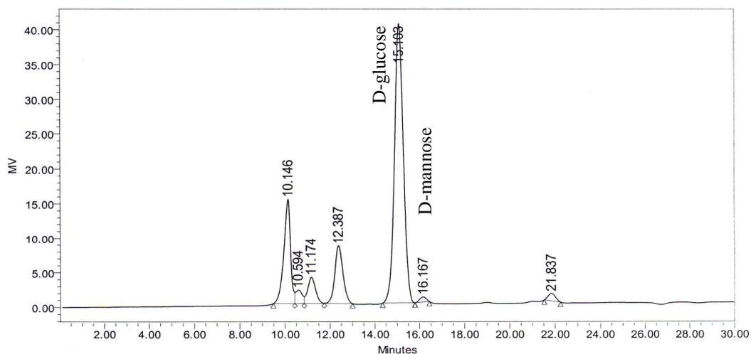
**Figure 6C.** HPLC Chromatogram of partial hydrolyzed exopolysaccharide from *Pediococcus* sp. P14 cultivated in MRS broth containing 2% of analytical grade sucrose with initial pH of 6.2 at 30°C. Sample injection volume was 100  $\mu$ l. Chromatographic run time was 30 min.
