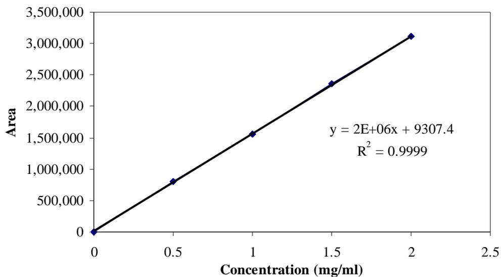
**Figure 5B.** Standard curve of white sugar from sugar cane using Vertisep™ OA HPLC with a 0.005 M H<sub>2</sub>SO<sub>4</sub> mobile phase and a refractive index detector.
