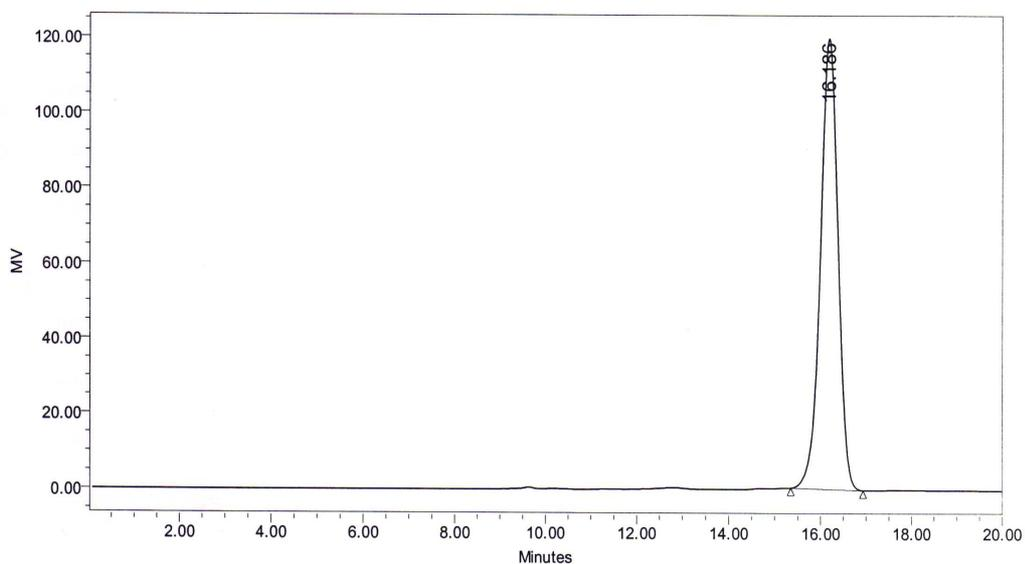
**Figure 13C.** HPLC Chromatogram of 2 mg/ml standard D-mannose using Vertisep™ OA HPLC with a 100% water mobile phase and a refractive index detector.
