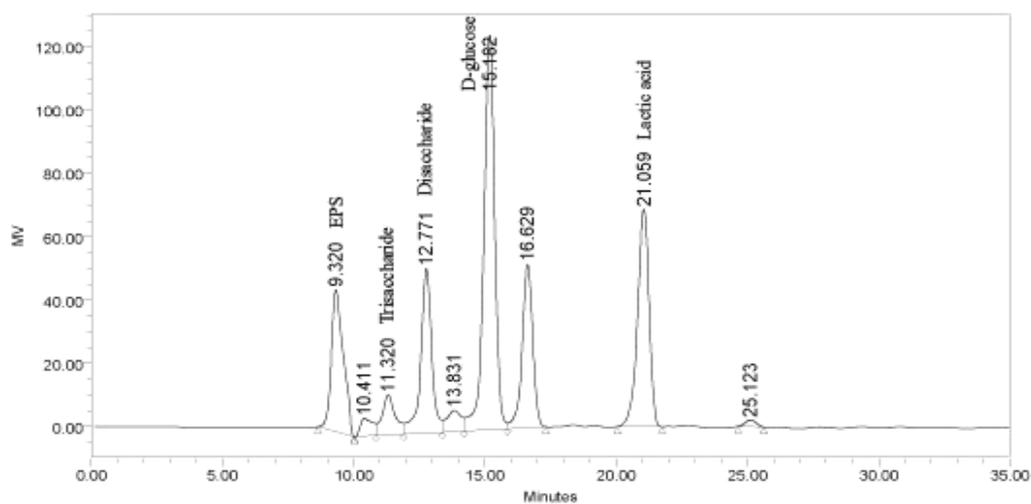
**Figure 16C.** HPLC Chromatogram of EPS, white sugar from sugar cane and lactic acid in culture broth using Vertisep™ OA HPLC with a 0.005M H<sub>2</sub>SO<sub>4</sub> mobile phase and a refractive index detector.
