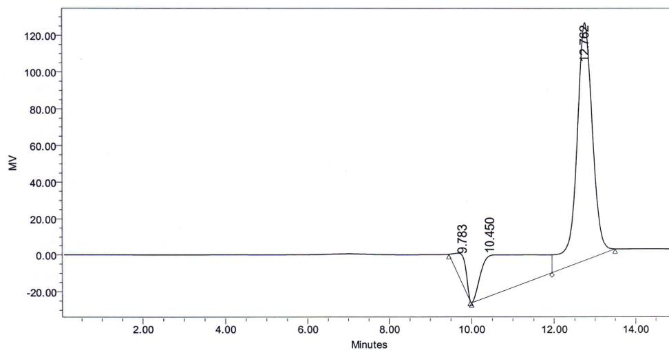
**Figure 12C.** HPLC Chromatogram of 2 mg/ml white sugar from sugar cane using Vertisep™ OA HPLC with a 0.005M H<sub>2</sub>SO<sub>4</sub> mobile phase and a refractive index detector.
