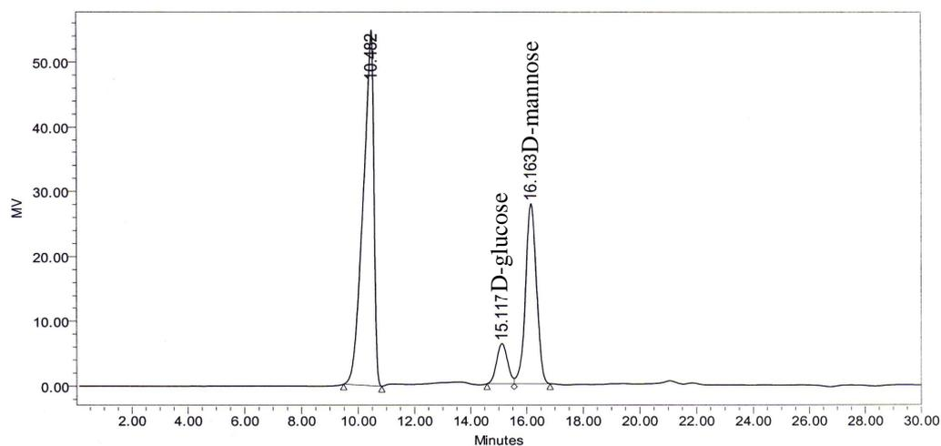
**Figure 3C.** HPLC Chromatogram of partial hydrolyzed exopolysaccharide from *Streptococcus* sp. G3 cultivated in MRS broth containing 2% of white sugar from sugar cane with initial pH of 6.2 at 30°C. Sample injection volume was 100  $\mu$ l. Chromatographic run time was 30 min.
