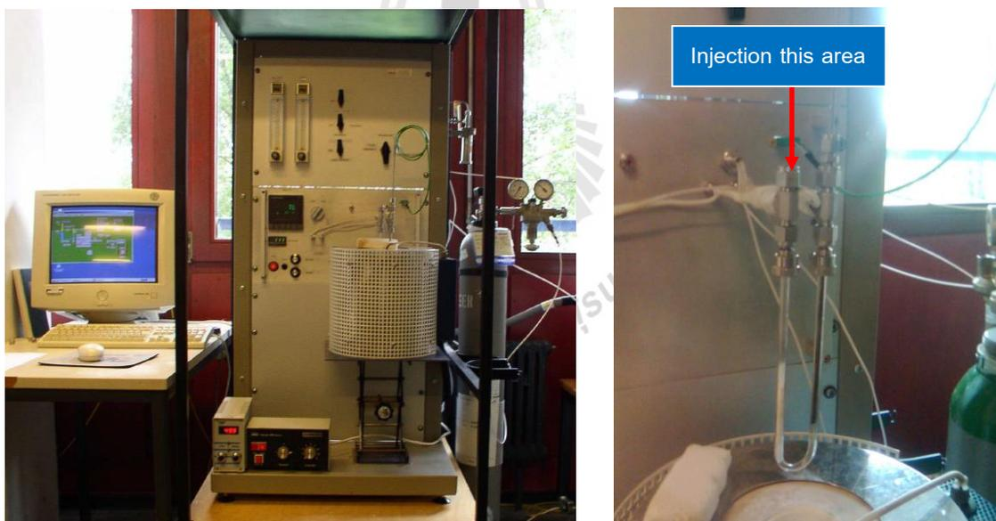
**Figure D.1** The apparatus for the study of TPD-pyrrole.
