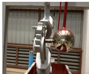
Fig. 3 Voltage Energized via Stainless Rod and Stainless Sphere
