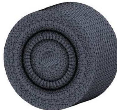
Fig. 2 Discretization of the induction motor
