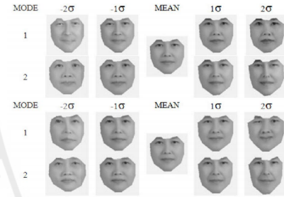
Fig 4 Appearance Models built from PCA (top) and ICA (bottom)
